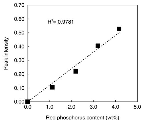
**Fig. 7.** Quantitative evaluation of red phosphorus using pyrolysis-gas chromatography/mass spectrometry
