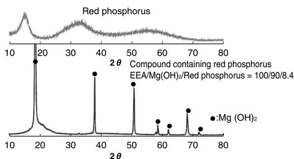
Fig. 3. X-ray diffractometry results of red phosphorus and compound containing red phosphorus
