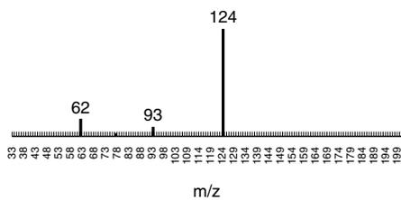
**Fig. 5.** Mass spectra of red phosphorus (peak ① in Fig. 4)
