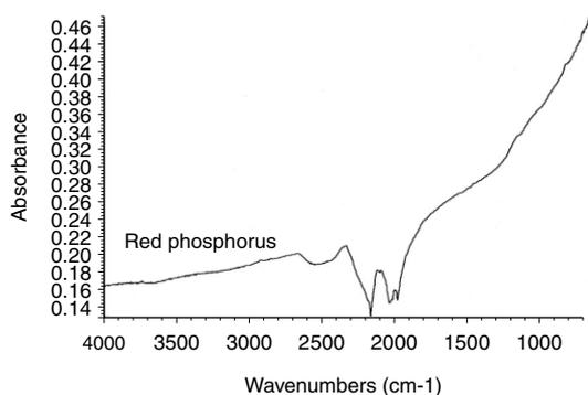
Fig. 1. Infrared absorption spectrum of red phosphorus
