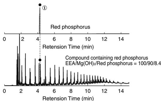
**Fig. 4.** Pyrolysis-gas chromatograms of red phosphorus and compound containing red phosphorus
