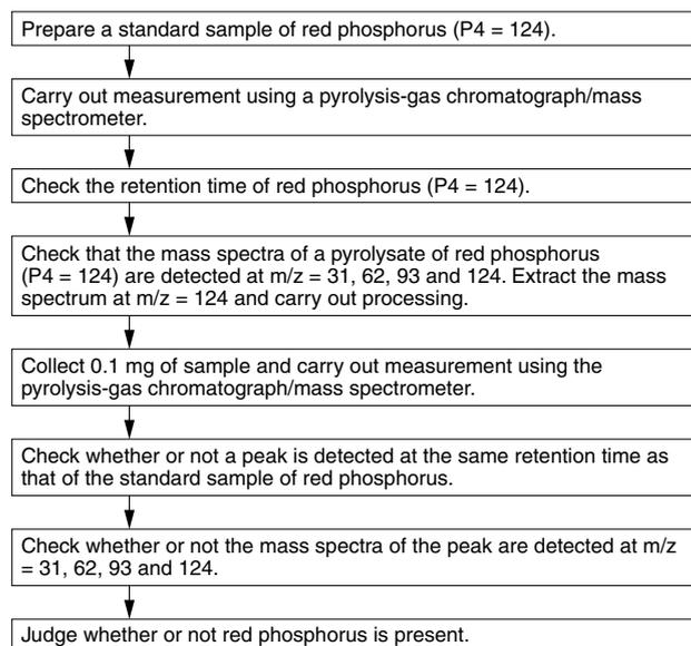
**Fig. 6.** Flowchart of analysis of red phosphorus in resins
