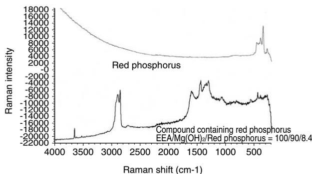
Fig. 2. Raman spectra of red phosphorus and compound containing red phosphorus
