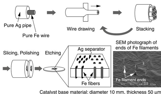
**Fig. 5.** Fabrication process of CTM catalyst
