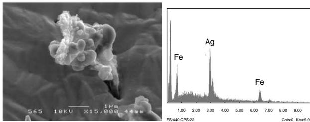
Fig. 7. (a) SEM image and EDX analysis of carbon substance
