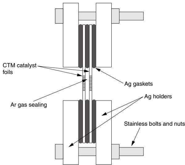
Fig. 6. Structure of specimen holder for CTM catalyst
