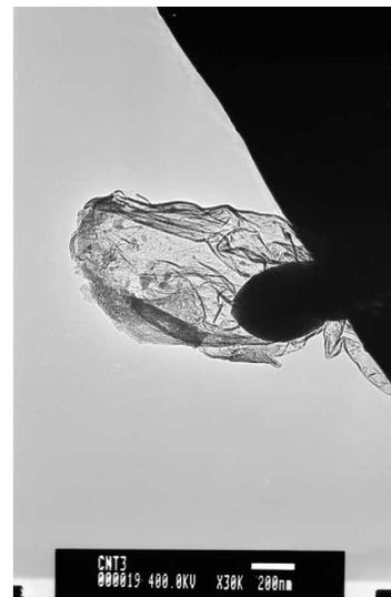
Fig. 8. TEM photograph of CNT generated at end of Fe filament at carbon transmission side
