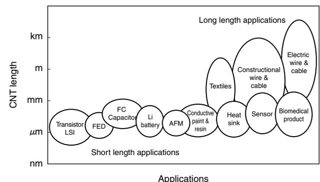
**Fig. 2.** Required CNT lengths for various applications
