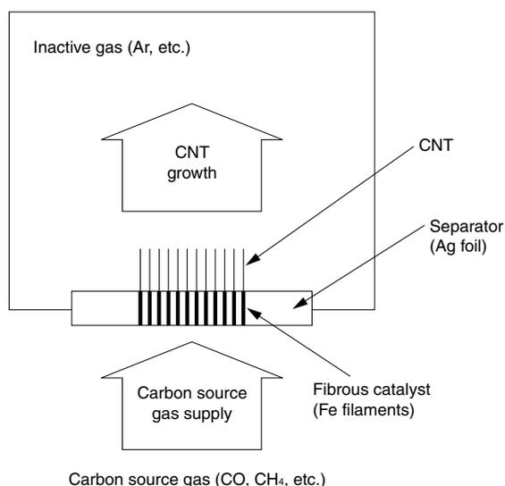
**Fig. 4.** Conceptual diagram of CNT growth by CTM process
