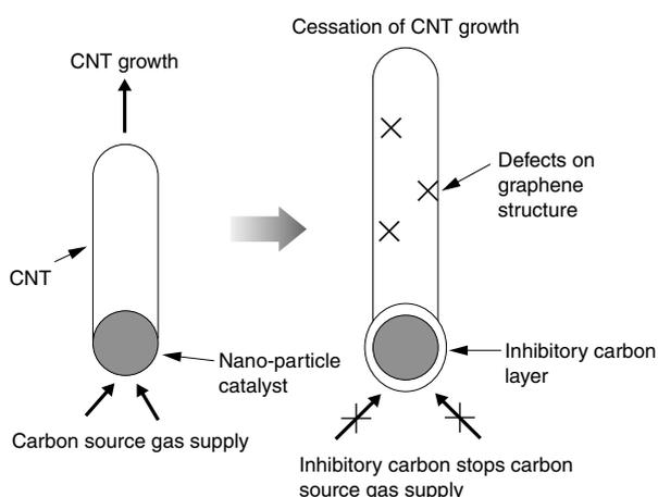
**Fig. 3.** Mechanism of growth and cessation of growth of CNT in thermal CVD process
