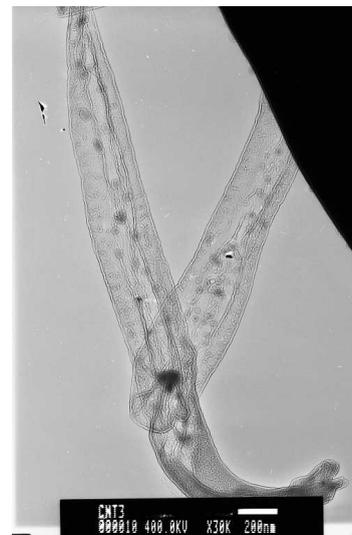
Fig. 9. TEM photograph of CNTs generated at carbon transmission side
