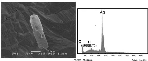
Fig. 7. (b) SEM image and EDX analysis of carbon nano-filament
