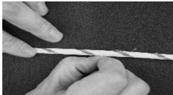
Photo 1. Holding wrapping tape with fingers
