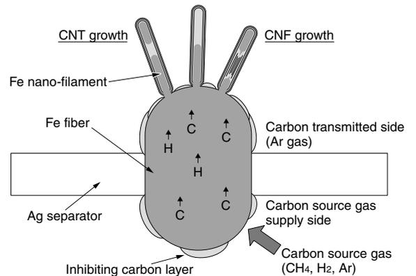
**Fig. 8.** Observed CNT growth mechanism of CTM process
