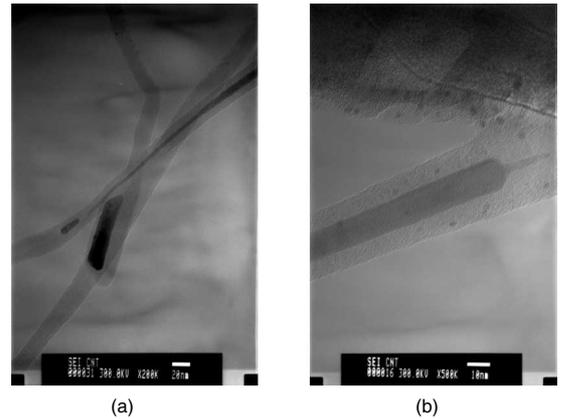
**Fig. 7.** TEM photographs of CNF with Fe nano-filament taken at (a) tip of Fe nano-filament and (b) base of Fe nano-filament
