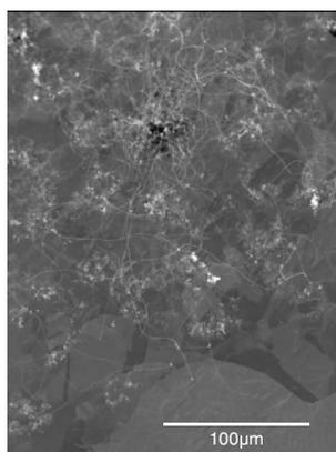
**Fig. 9.** SEM photograph of CNTs of over 100  $\mu\text{m}$  in length at carbon transmitted side of CTM catalyst foil specimen
