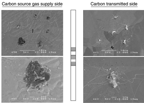
**Fig. 4.** SEM photographs of Fe fiber ends on CTM catalyst foil specimens after heat treatment of carbon materials
