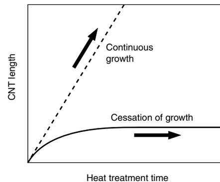
**Fig. 1.** Heat treatment time dependence of thermal CVD-grown CNT
