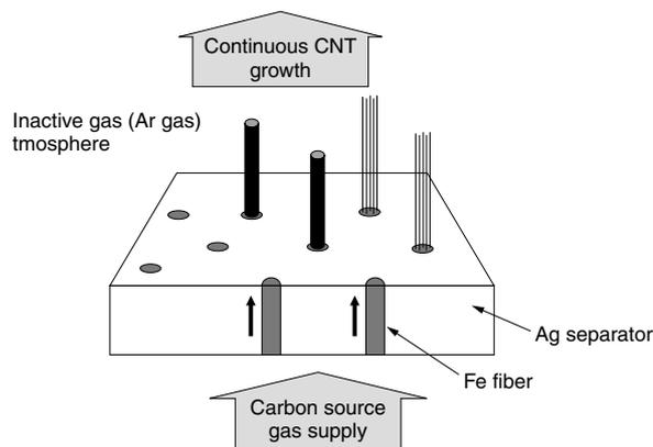
Fig. 2. Conceptual illustration of CNT growth using CTM process
