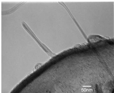
**Fig. 5.** TEM photograph of CNTs and CNFs by CTM process
