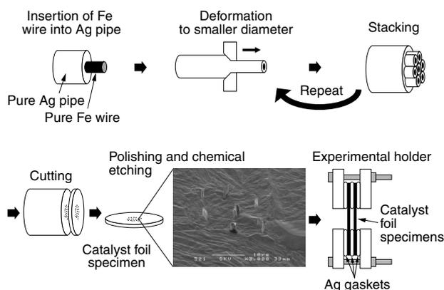
Fig. 3. Fabrication process of catalyst foil specimen for CTM
