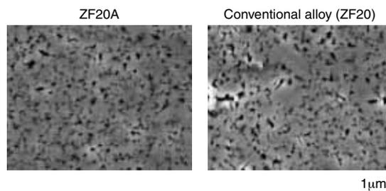
Photo 1. Microscopic structures of ZF20A and ZF20
