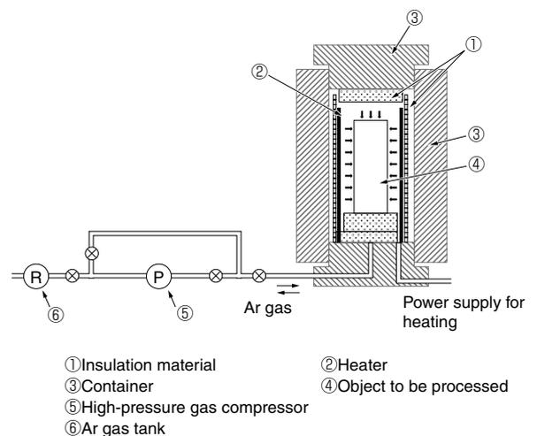
Fig. 6. Schematic view of HIP system
