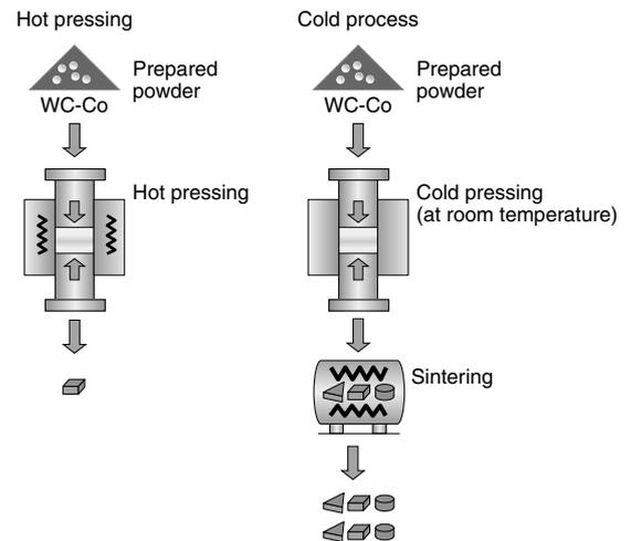
Fig. 3. Cemented carbide manufacturing methods (Hot pressing and cold process)
