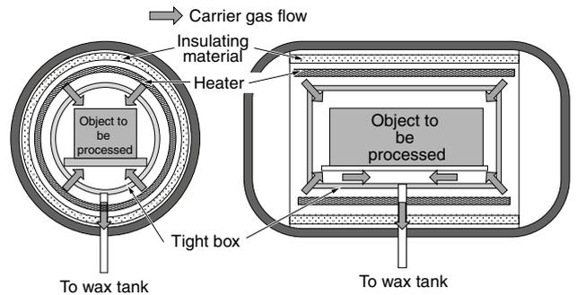
Fig. 5. Tight box structures
