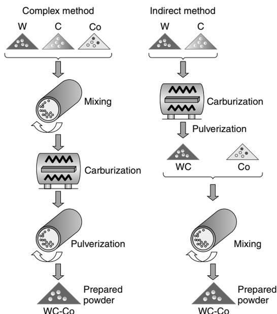
Fig. 2. WC-Co powder preparation methods (Complex method and indirect method)
