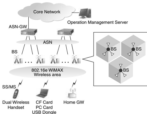
Fig. 6. WiMAX system configuration
