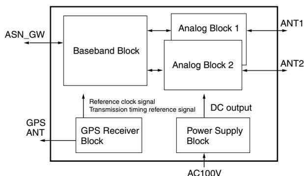
Fig. 1. Block diagram of prototype WiMAX base station
