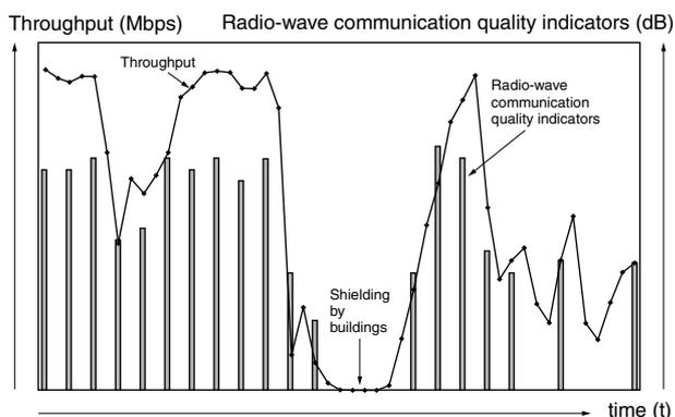
Fig. 8. Adaptive modulation measurement
