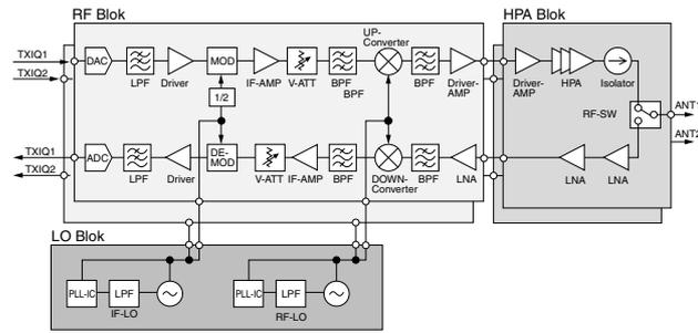
**Fig. 3.** Block diagram of analog block
