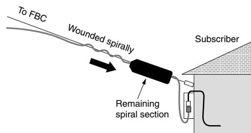
**Fig. 8.** Installation method for spiral drop cable
