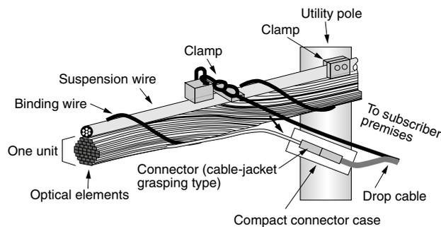
Fig. 3. Configuration of cable drop point
