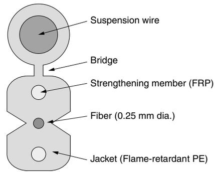
**Fig. 6.** Cross-section of spiral drop cable
