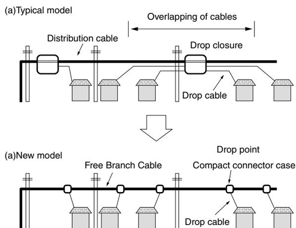
Fig. 1. Typical FTTH network model in Japan and new model
