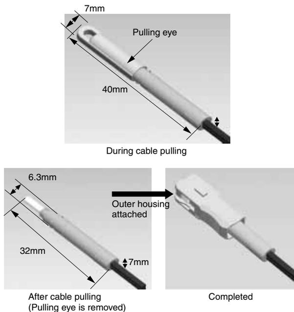
**Fig. 9.** Structure of slim connector
