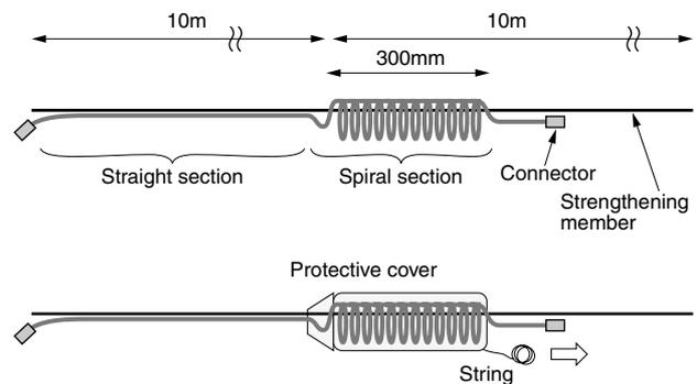
**Fig. 7.** Structure of spiral drop cable
