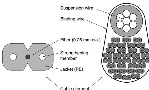
Fig. 2. Cross-section of FBC
