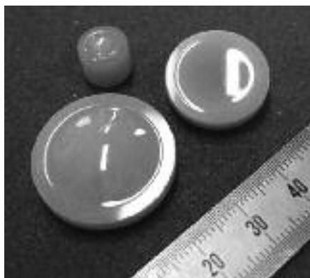
Photo 1. Developed ZnS lens
