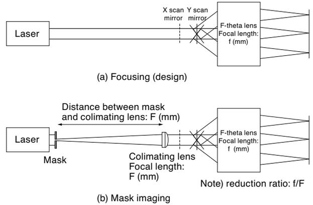
**Fig. 3.** Optical systems of typical laser drilling machine
