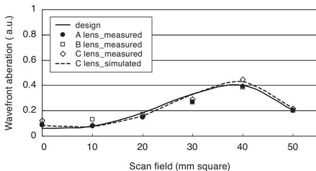
Fig. 8. Transmission wavefront measurement results
