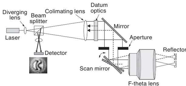
Fig. 7. Transmission wavefront measurement
