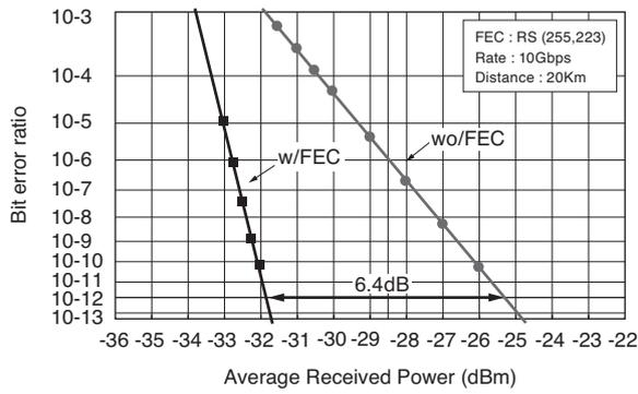
Fig. 6. BER Characteristics after FEC Decode
