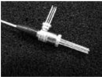
Fig. 4. ONU Bi-directional Device
