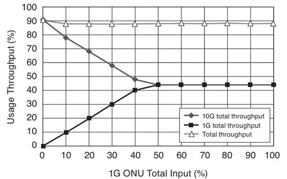
Fig. 8. Upstream Efficiency under Co-existence
