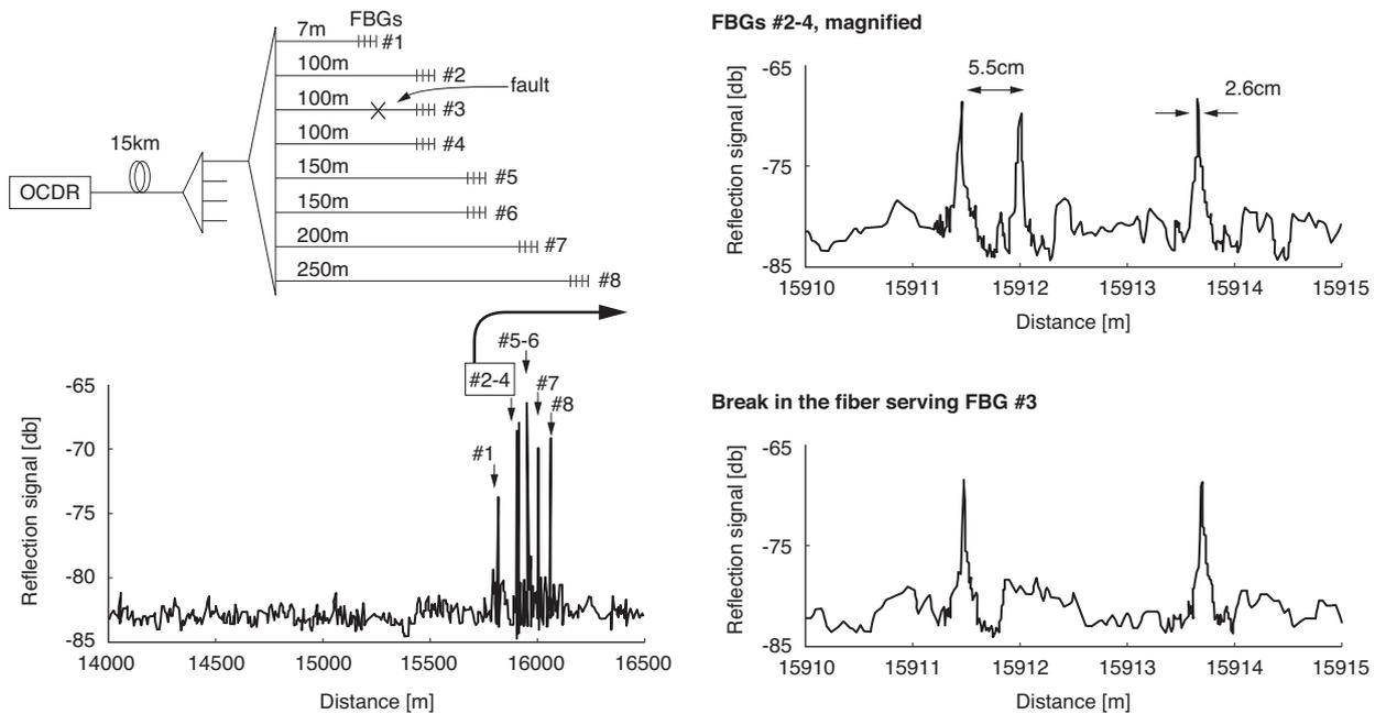
**Fig. 2.** Experimental results. Reflections from FBGs below 32 branch at 15km distance are detected. Spatial range is 2.6km and spatial resolution is 2.6cm. When a fiber-breaking fault is simulated by disconnecting FBG #3, the fault is detected as an absence of reflection peak
