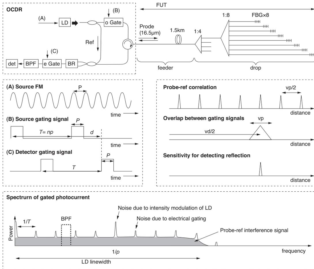
Fig. 1. Schematic diagram of pulse-OCDR. LD: laser diode, oGate: optical gate, FUT: fiber under test, BR: balanced receiver, eGate: electrical gate, BPF: band-pass filter, det: RF detector, FBG: fiber Bragg grating reflecting 1.65 $\mu\text{m}$ ,  $p$ : period of frequency modulation,  $T$ : period of gating signals,  $n$ : an integer,  $d$ : delay between the source and detector gating signals,  $v$ : group velocity of light in the fiber
