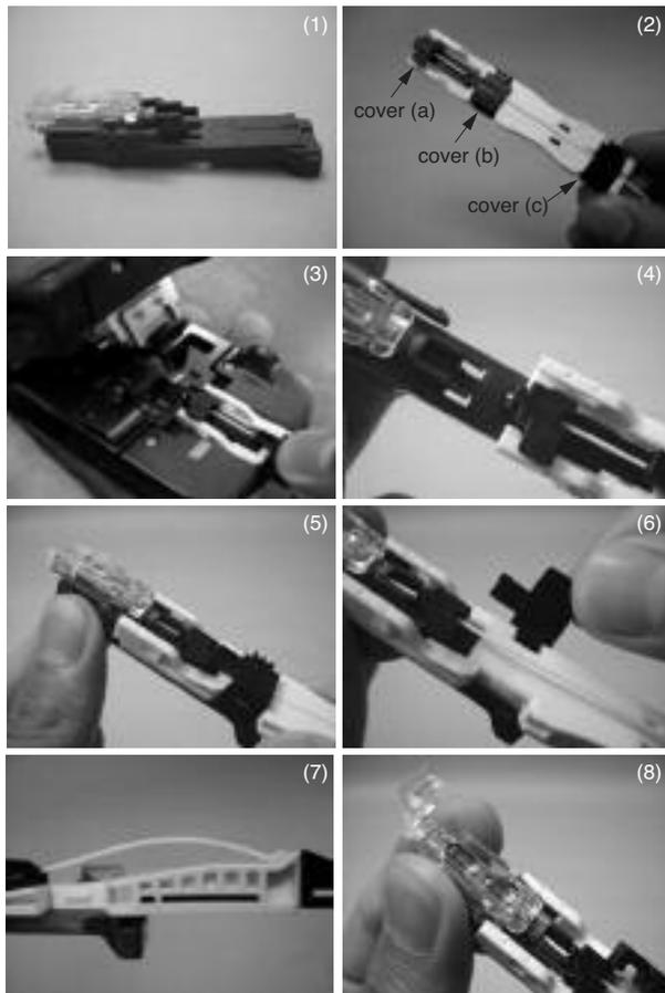
Photo 4. Outline of assembly procedure of LC connector for ø0.9 mm fiber
