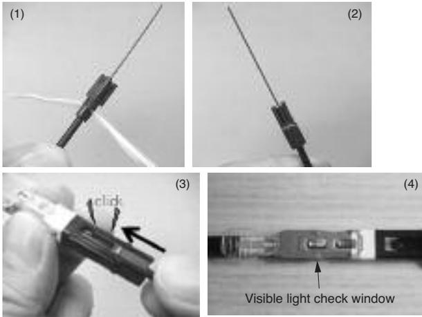
**Photo 2.** Outline of assembly procedure of field assembly connector for ø3 mm cord
