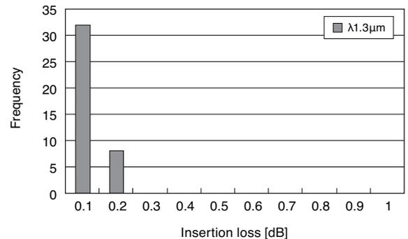
Fig. 5. Insertion loss distribution of assembled connectors for ø0.9 mm fiber by amateur worker
