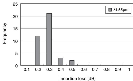
**Fig. 4.** Insertion loss distribution of field assembly connectors for ø3 mm cord (SM type)
