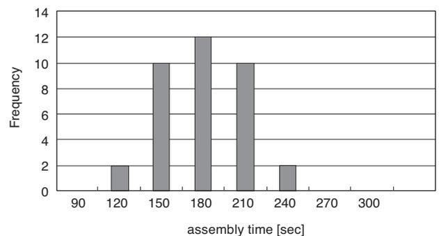
Fig. 6. Working time of connectors for ø0.9 mm fiber (MM50 type) by amateur worker
