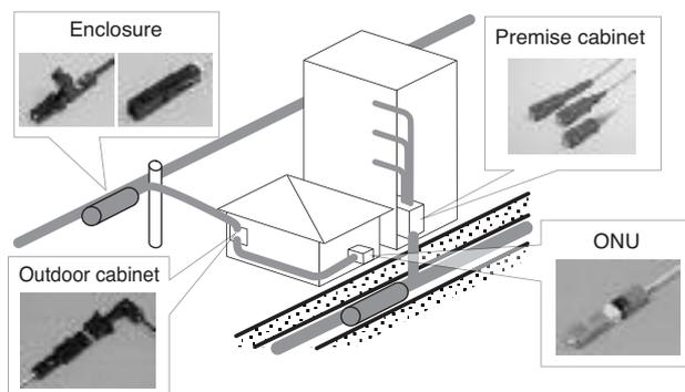
Fig. 1. Application domain of field assembly connectors in Japan
