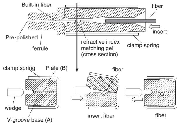
Fig. 3. Fundamental structure and mechanism of mechanical splice
