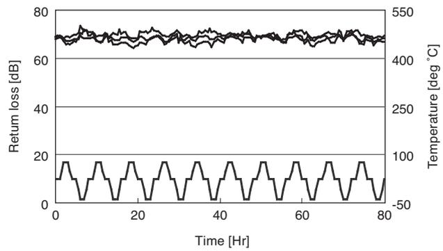
**Fig. 7.** Return loss properties of field assembly angled polishes SC connectors for 0.9 mm fiber at heat cycle test
