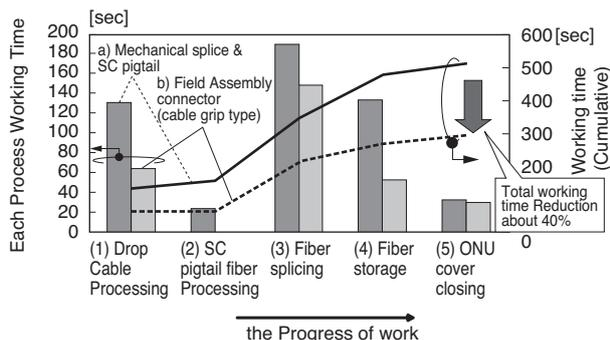
Fig. 2. Comparison of working time of fiber installation at ONU (Mechanical splice vs Field Assembly connector)
