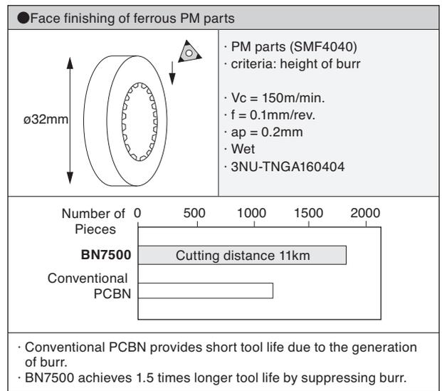
Conventional PCBN provides short tool life due to the generation of burr.
