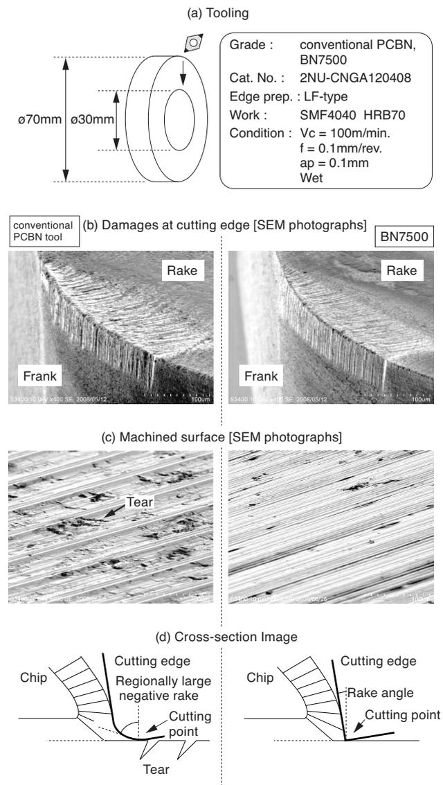
Fig. 4. Results of cutting test of white turbidity on ferrous PM
