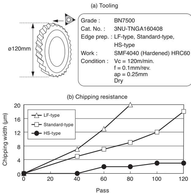
Fig. 3. Results of cutting test on hardened ferrous PM
