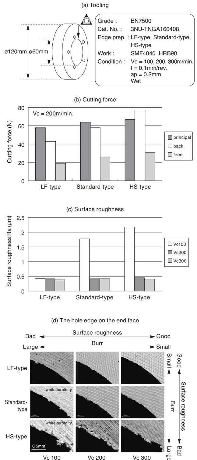
**Fig. 2.** Results of cutting test on standard ferrous PM
