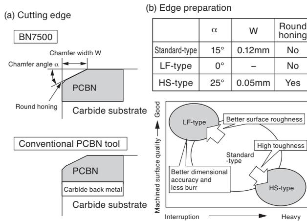
**Fig. 1.** Structure of the cutting edge of BN7500
