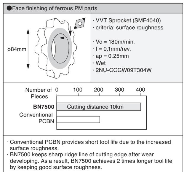
Conventional PCBN provides short tool life due to the increased surface roughness.
