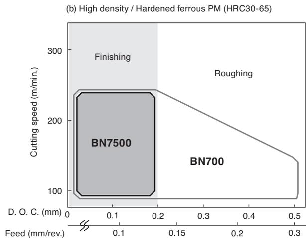
Wet cutting is recommended for continuous cutting of standard ferrous PM parts. Dry cutting is recommended for interrupted cutting of hardened ferrous PM parts.
