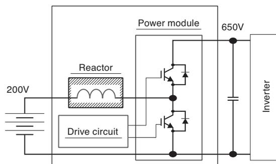
Fig. 2. Example of the boost converter
