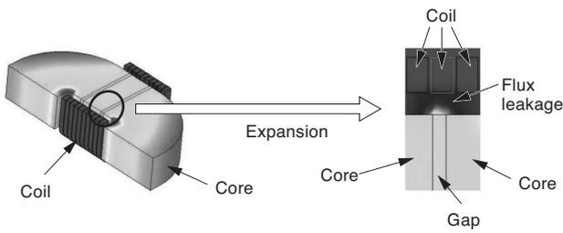
Fig. 8. Contour figure of electromagnetic field analysis
