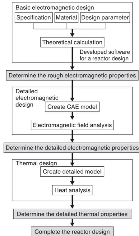
Fig. 3. Process of designing a reactor
