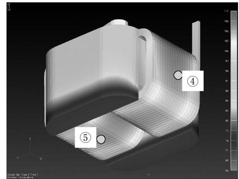
**Fig. 15.** Measurement point of the reactor temperature
