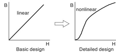
Fig. 7. Nonlinear magnetic properties
