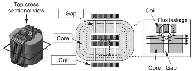
Fig. 6. Flux leakage from the gap
