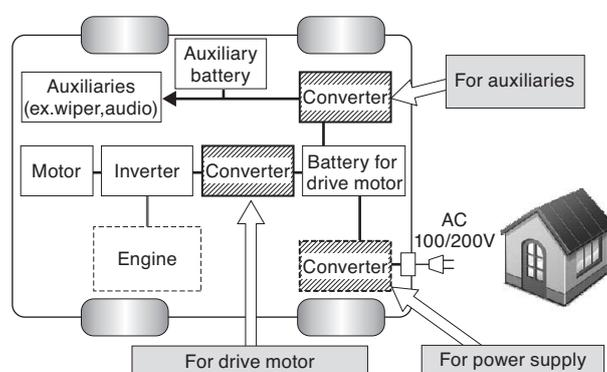
Fig. 1. HEV, PHEV, EV Systems
