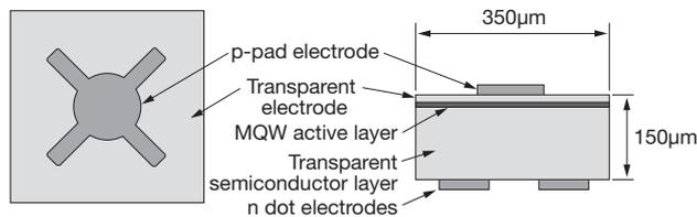
**Fig. 1.** 940 nm infrared LED structures
