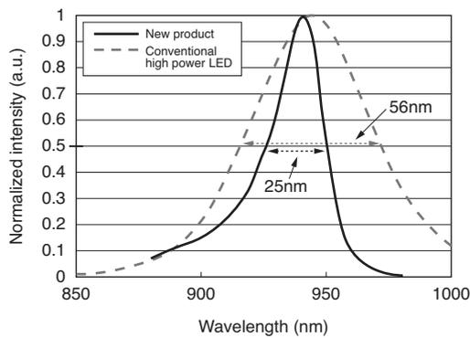
Fig. 4. Light emission spectrum of 940 nm infrared LED
