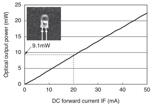
**Fig. 3.** Current-light output power characteristics of a 5 mmø bullet LED lamp
