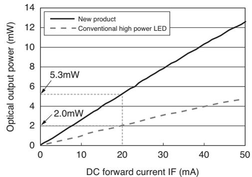
**Fig. 2.** Current-light output power characteristics of a 940 nm infrared LED
