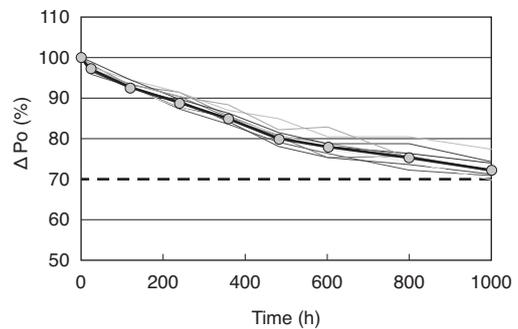
Fig. 6. Accelerated life time testing results of 940 nm infrared LEDs
