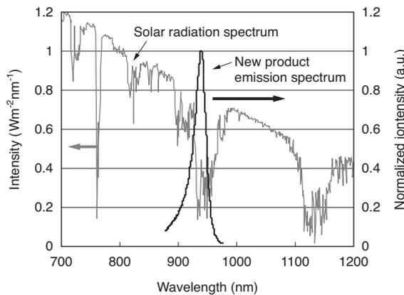
Fig. 5. Light emission spectrum of 940 nm infrared LED and solar radiation spectrum
