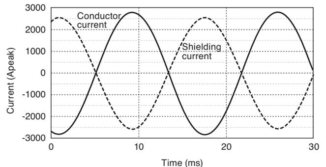
Fig. 9. Waveform of HTS shielding current at loading current of 2 kArms
