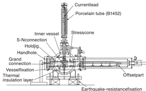
**Fig. 5.** Schematic view of “3-in-One” HTS termination
