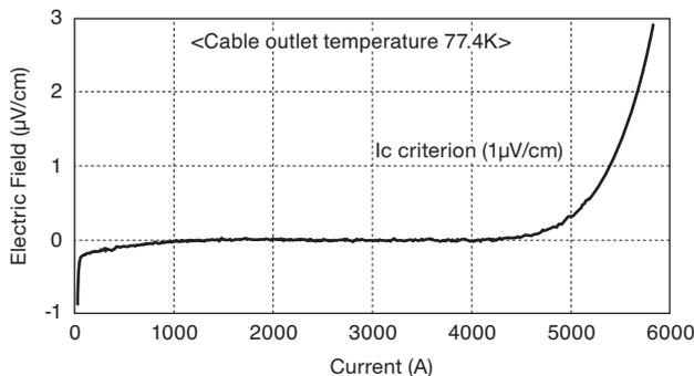
Fig. 8. Analyzed I-E characteristics of cable conductor
