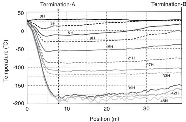
Fig. 7. Temperature profiles of 1<sup>st</sup> step initial cooling
