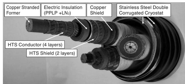
**Photo 1.** Structure of “3-in-One” HTS cable
