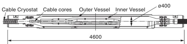
**Fig. 4.** Schematic view of “3-in-One” HTS joint
