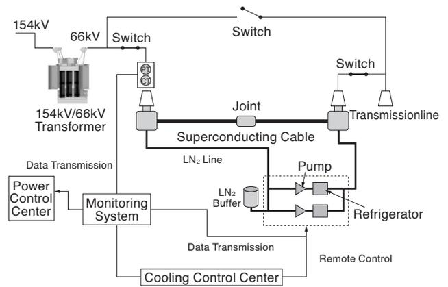
**Fig. 1.** Configuration of the demonstration system in Asahi substation
