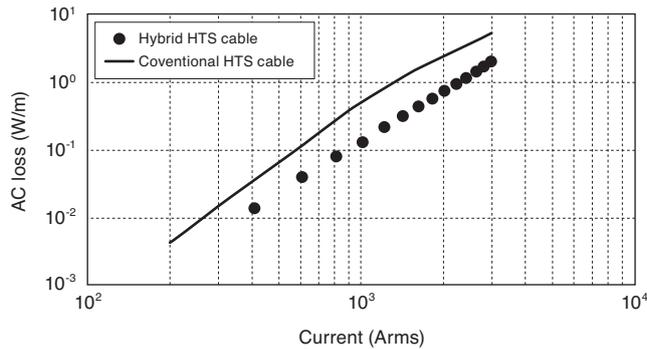
Fig. 2. AC loss test results for hybrid HTS cable core
