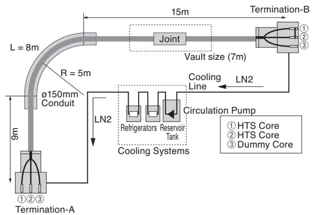
**Fig. 6.** 30-meter HTS cable system configuration
