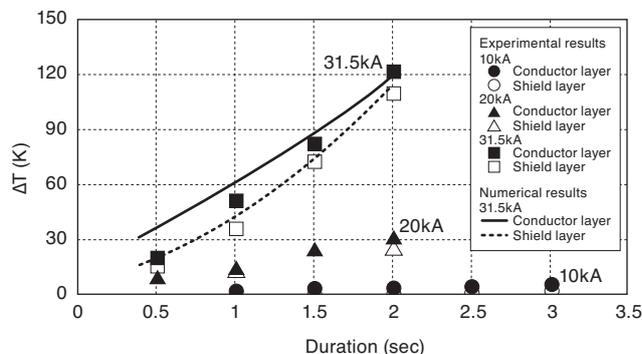
Fig. 3. Fault current test results of HTS cable core
