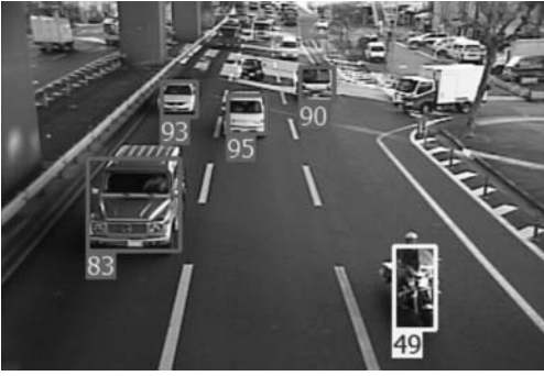
Fig. 8. Result of cooperation of the vehicle detection and vehicle tracking Figures at the lower left show the identification number specific to each tracked vehicles or motorcycles
