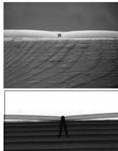
Photo 2. Appearance of stapled (top) PureFlex-slim and its X-ray photograph (bottom).
