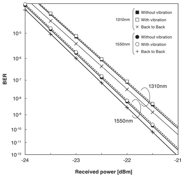
Fig. 12. Bit error rate under 10 Gbps transmission with or without applying vibration
