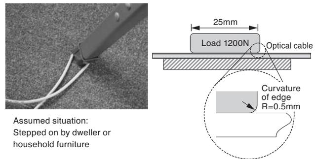
Fig. 8. Apparatus of crush test and assumed situation
