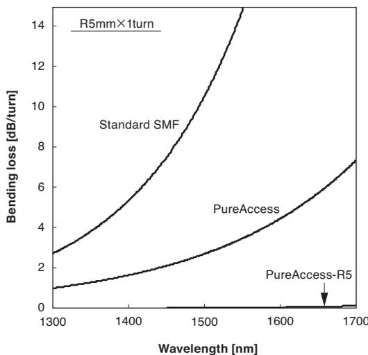
**Fig. 1.** Comparison of wavelength dependence of bending loss
