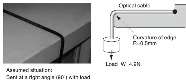
Fig. 10. Apparatus of L-bend test and assumed situation
