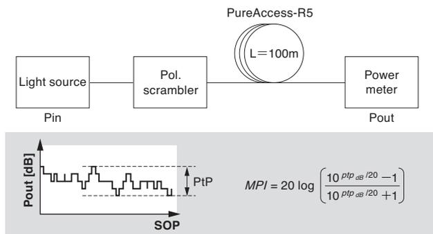
Fig. 6. Measurement setup of MPI
