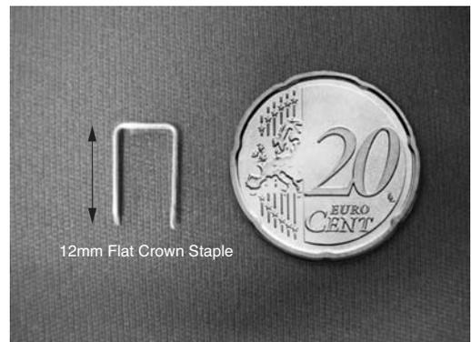
Photo 1. Flat staple used in the test
