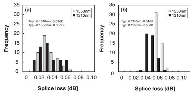
**Fig. 2.** Fusion splice loss between (a) PureAccess-R5 to PureAccess, (b) PureAccess-R5 to standard SMF
