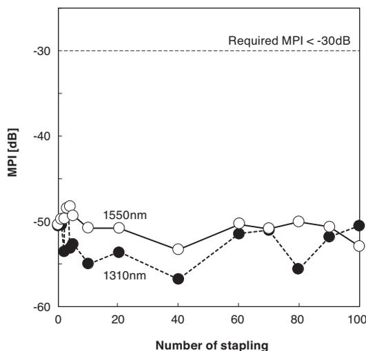
Fig. 7. Change in measured MPI by stapling
