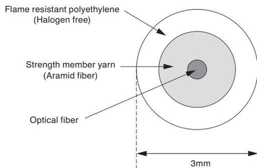
Fig. 4. Cross section of PureFlex-slim cable
