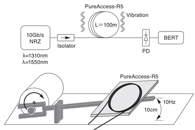
**Fig. 11.** Bit error rate measurement setup under fiber vibration
