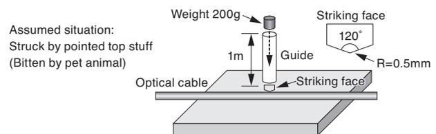
Fig. 9. Apparatus of impact test and assumed situation
