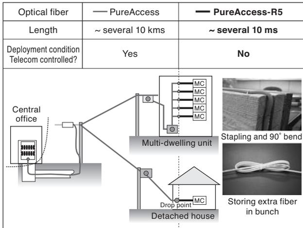
Fig. 3. FTtx deployment example using PureAccess-R5 and PureAccess
