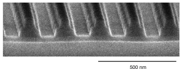
**Fig. 5.** Cross-sectional SEM image of gratings after the penetration etching of the resin.
