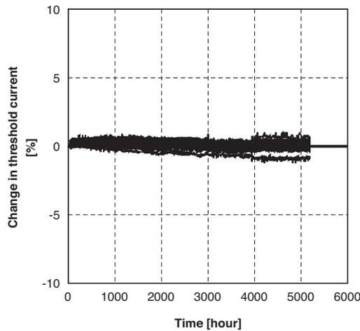
**Fig. 11.** Time-dependent change in threshold current of phase-shifted DFB LDs with the output power of 10 mW at the ambient temperature of 85°C.
