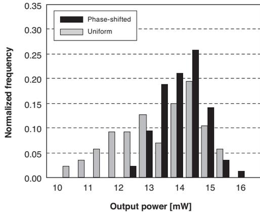
**Fig. 10.** Histograms of maximum output power for phase-shifted LDs and uniform-grating LDs fabricated by NIL. The standard deviations of output power for phase-shifted LDs and uniform-grating LDs are 0.74 and 1.27, respectively.
