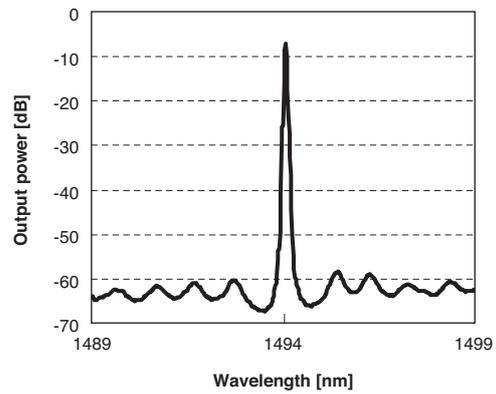
Fig. 8. Oscillation spectrum of a phase-shifted LD.
