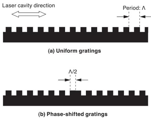
Fig. 2. Schematic structures of uniform gratings (a) and phase-shifted gratings (b).
