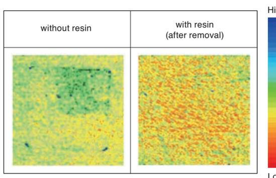
**Fig. 4.** Comparison of photoluminescence intensities between two samples: imprinted without resin (left) and imprinted with resin (right). The field size of imprinting is 10 mm × 10 mm.
