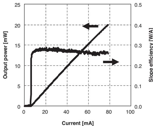
Fig. 7. Supplied current vs. optical output and slope efficiency.
