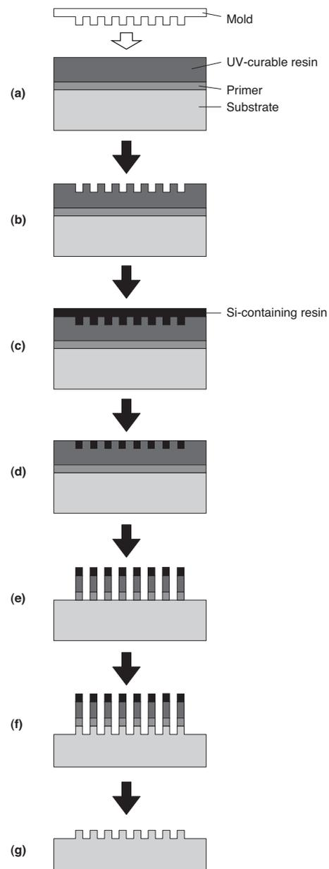
Fig. 3. Fabrication process of diffraction gratings.
