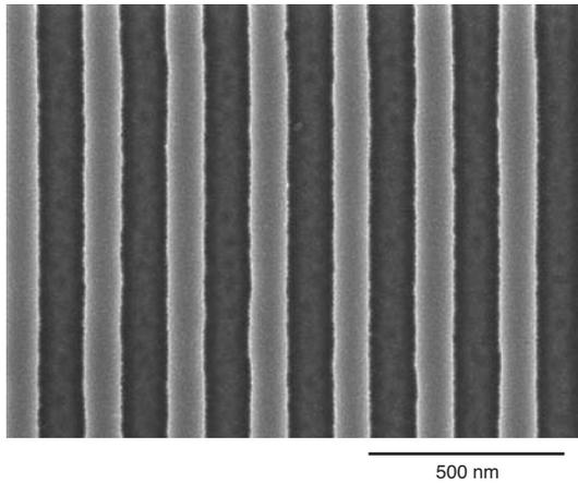
Fig. 6. SEM image of diffraction gratings after the crystal etching.
