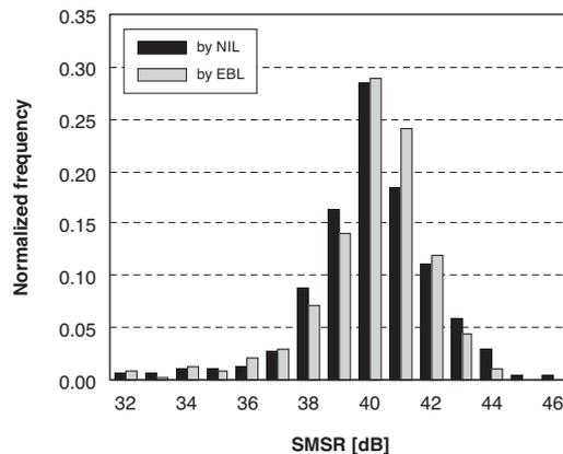
Fig. 9. Histograms of SMSR for phase-shifted LDs fabricated by NIL and by EBL. The standard deviations of SMSR for LDs fabricated by NIL and by EBL are almost the same, 2.0 and 1.8, respectively.
