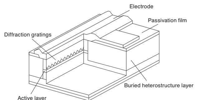
Fig. 1. Schematic structure of a DFB LD.
