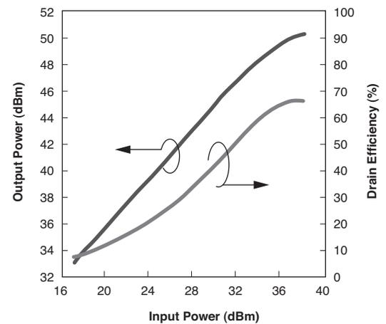
Fig. 3.  $P_{in}$ - $P_{out}$  profile of 100 W class GaN HEMT
