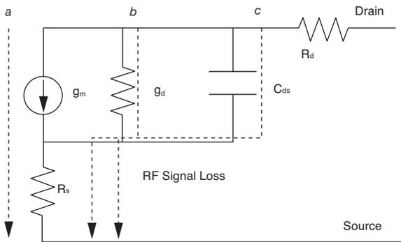
Fig. 4. Power dissipation path of GaN HEMT
