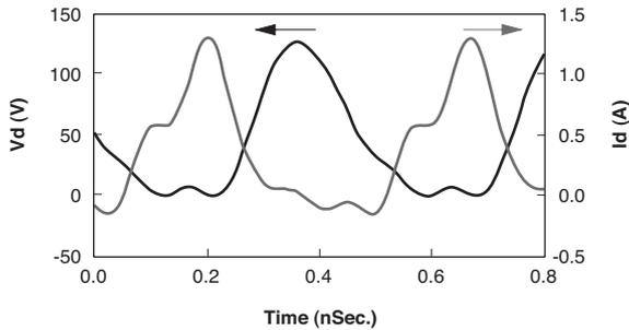
Fig. 11. Simulated waveform of low pass type Class-E amplifier at  $P_{out} = 10$  W,  $V_{ds} = 50$  V, freq. = 2.1 GHz
