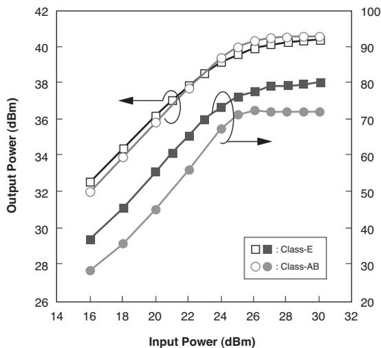
Fig. 12.  $P_{in}$ - $P_{out}$  of Class-E amplifier
