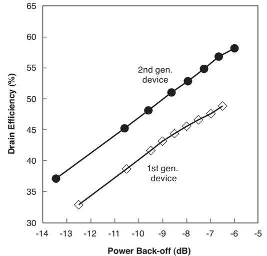
Fig. 9. Drain efficiency comparison of Doherty PAs with 1st gen. and 2nd gen. tech
