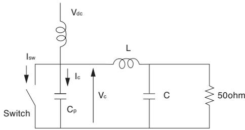
Fig. 10. Low pass type Class-E circuit
