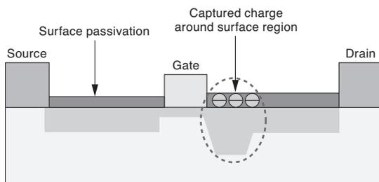
Fig. 1. Schematic image of current collapse
