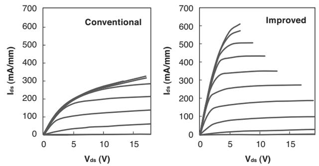
Fig. 2. Pulsed I-V profile of conventional and improved chip
