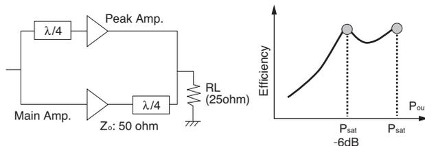
Fig. 8. Schematic of Doherty PA and efficiency profile
