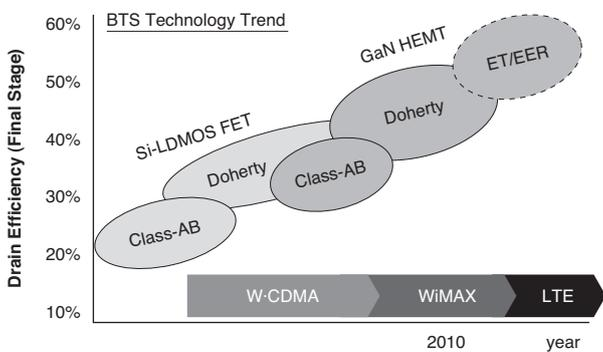
Fig. 5. BTS technology trend and required drain efficiency
