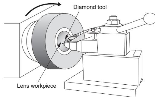
Fig. 9. Lens machining with ultraprecision lathe
