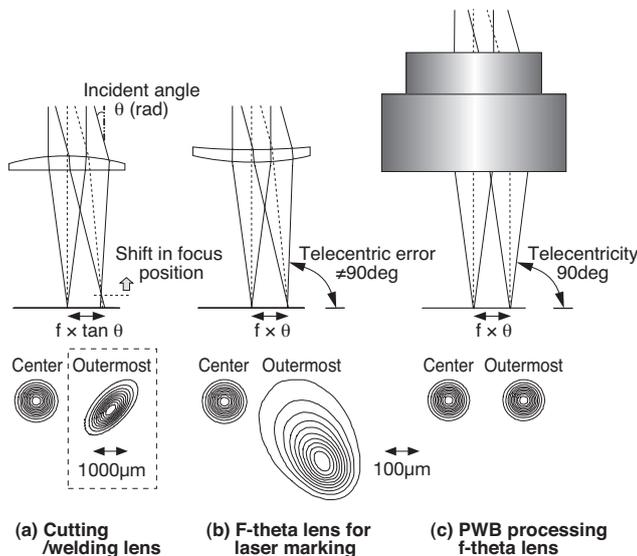
**Fig. 3.** Comparison of laser processing lens characteristics (Entry of 13 mm diameter Gaussian beam, with 9.4  $\mu\text{m}$  wavelength and 100 mm focal length)
