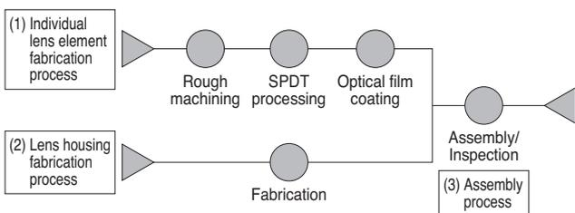
Fig. 8. F-theta lens fabrication flow
