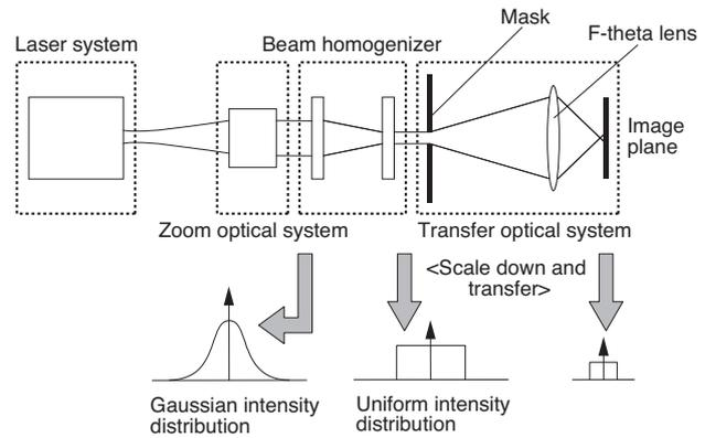
Fig. 12. Taperless hole drilling optical system
