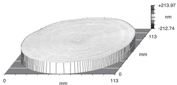
Fig. 10. Figure accuracy of ZnSe aspheric lens
