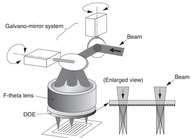
Fig. 13. Multi-hole drilling optical system
