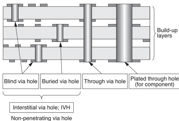
Fig. 1. Build-up board with via holes
