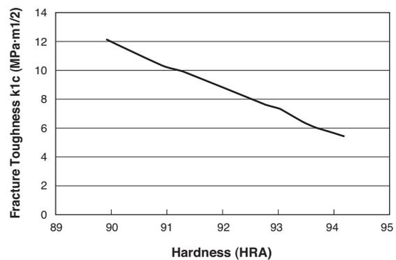
Fig. 9. Relation between hardness and fracture toughness
