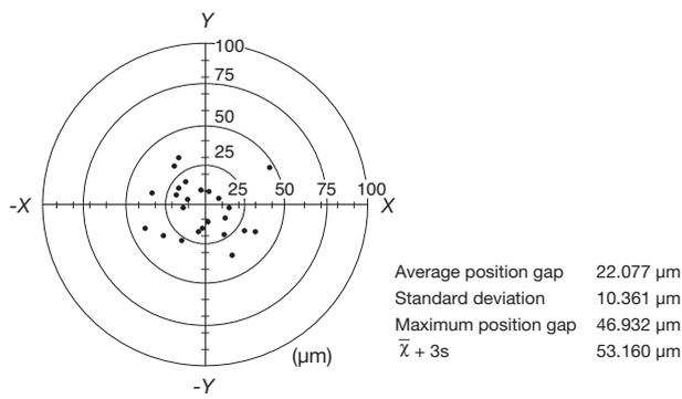
Fig. 6. Measurement of hole positioning accuracy
