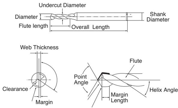
Fig. 2. Figures and names of microdrill parts
