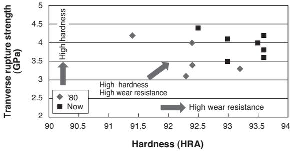
Fig. 10. Development of microdrill materials
