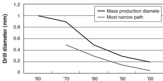
Fig. 3. Shifts in microdrill diameters
