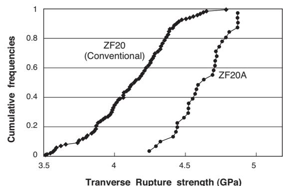
Fig. 12. Transverse rupture strength of ZF20A
