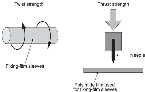
Fig. 3. Twist strength and thrust strength
