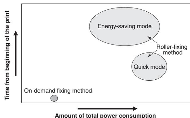
Fig. 2. Relation between time from beginning of the print and amount of total power consumption
