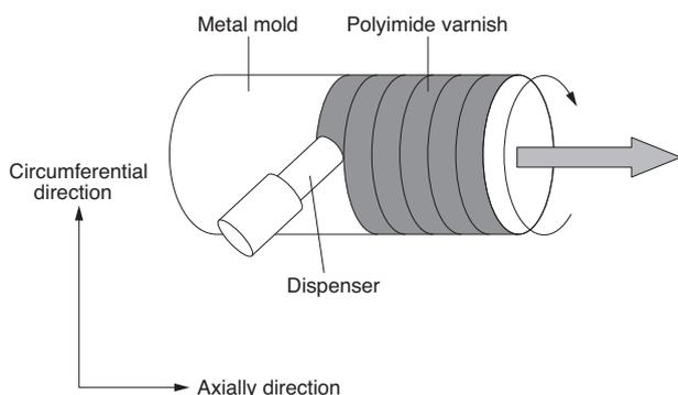
**Fig. 8.** Spreading method of polyimide varnish
