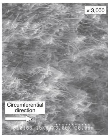
**Photo 1.** Cross section of fixing-film sleeve with CNF mixed
