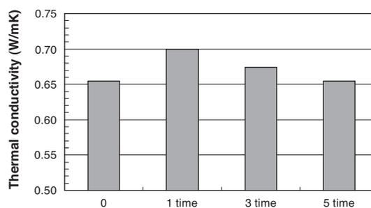
Fig. 6. Relation between processing frequency of roll milling and thermal conductivity
