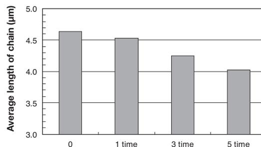
Fig. 7. Relation between processing frequency of roll milling and average length of CNF chain
