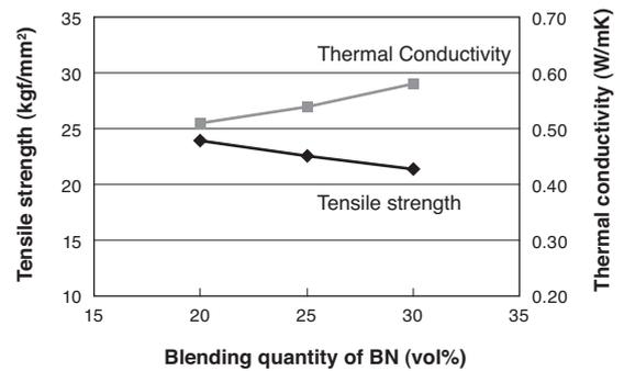
Fig. 4. Relation among BN blending quantity, tensile strength, and thermal conductivity
