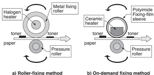
Fig. 1. Structure comparison between the roller-fixing method and the on-demand fixing method
