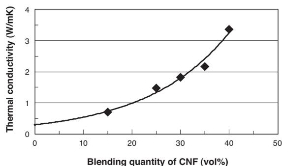
Fig. 5. Relation between blending quantity of CNF and thermal conductivity
