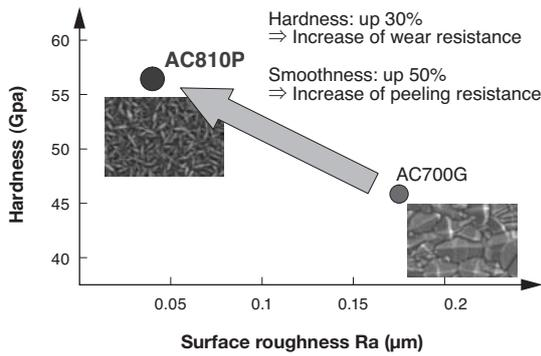
Fig. 5. Physical properties of Super FF-TiCN
