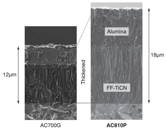
Fig. 3. Cross sectional SEM images of AC810P and conventional grade AC700G
