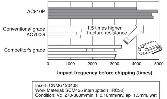
Fig. 7. Evaluation results on fracture resistance under interrupted cutting
