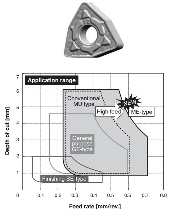
Fig. 8. Design and application range of newly developed ME-type for rough machining
