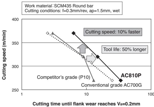
Fig. 6. Evaluation results on wear resistance under high speed machining
