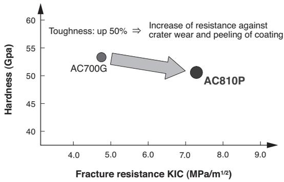
Fig. 4. Physical properties of newly developed alumina
