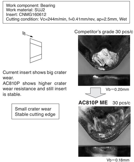
Fig. 11. Trial experiment of the combination of AC810P and ME-type
