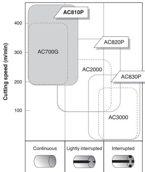
Fig. 2. Application domains of AC810P, AC820P and AC830P
