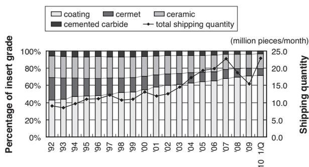
Fig. 1. Proportion of each indexable insert grade in total shipping quantity (Japan)<sup>(1)</sup>
