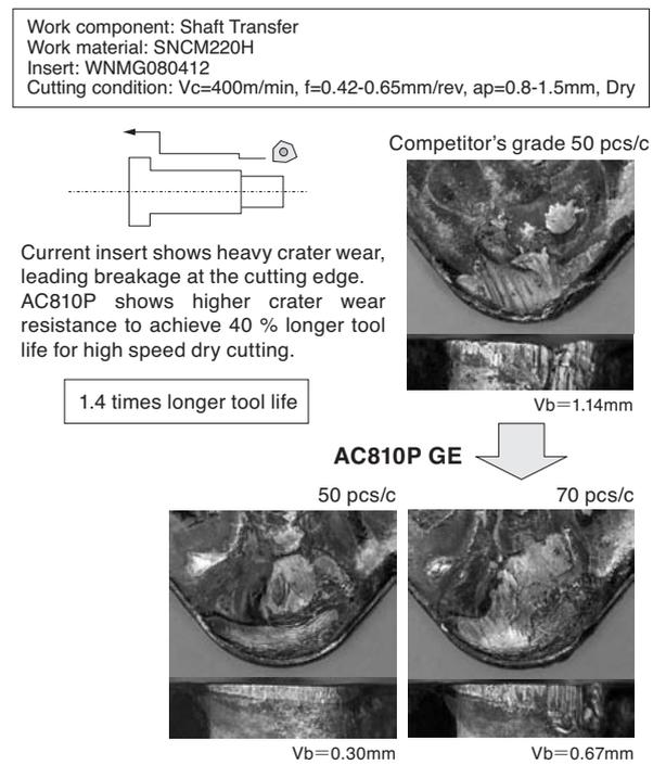
Fig. 10. Trial experiment of AC810P for high speed and dry cutting
