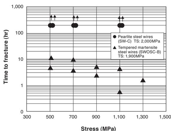
Fig. 1. Delayed Fracture Properties Comparison between Pearlite Steel and Tempered Martensite Steel
