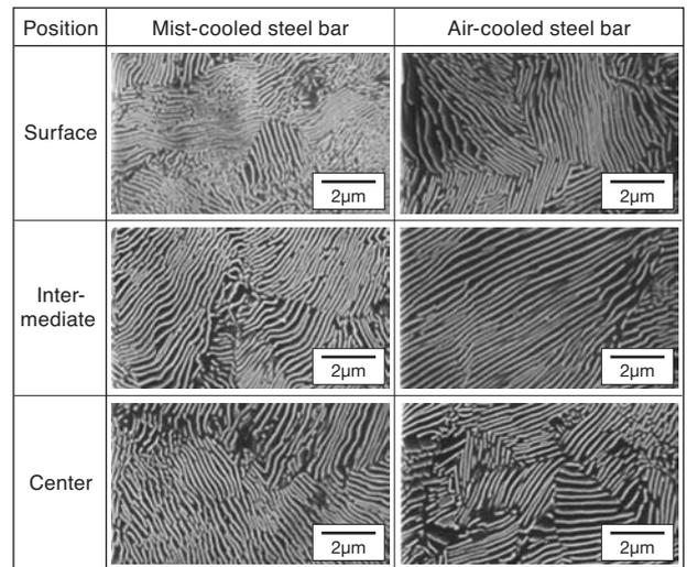
**Photo 3.** Pearlite Lamella Structures by SEM
