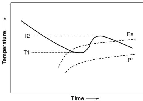
Fig. 2. Schematic Illustration of Cooling Curve
