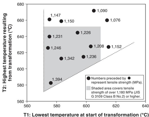
Fig. 3. Relation between Pearlite Transformation Temperature and Tensile Strength
