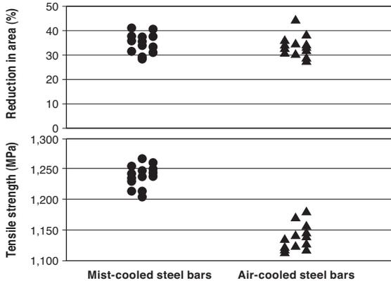
Fig. 6. Mechanical Properties of Steel Bars
