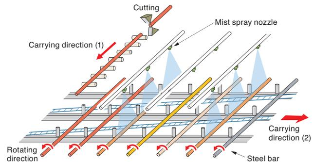
Fig. 4. Schematic Illustration of Steel Bar Mist-Cooling System
