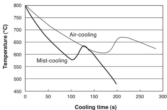
**Fig. 5.** Cooling Curve for Steel Bars
