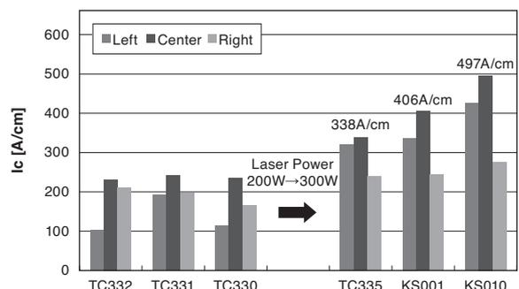
Fig. 5. Increase in I<sub>c</sub> values of 30 mm-width Clad-PLD conductors
