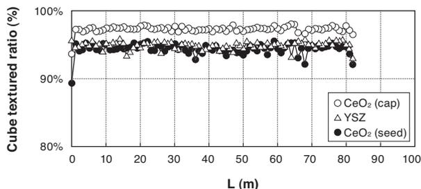
Fig. 2. Longitudinal cube-textured characteristics of CeO<sub>2</sub>/YSZ/CeO<sub>2</sub> long buffer layer
