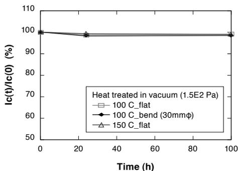
**Fig. 9.** Time duration of  $I_c$  property under vacuum condition
