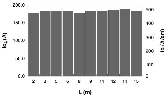
Fig. 6. Longitudinal  $I_c$  distribution of 4 mm-width Clad-PLD conductor
