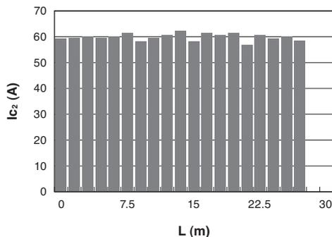
Fig. 7. Longitudinal  $I_c$  distribution of 2 mm-width Clad-PLD conductor
