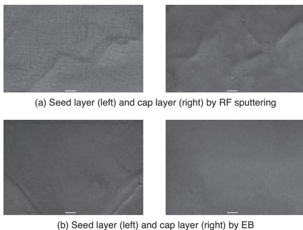
Fig. 3. Improvement of surface morphology of buffer layers by using EB evaporation method
