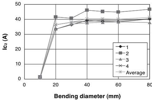
Fig. 12. Bending stress effect on the  $I_c$  of Clad-PLD conductor
