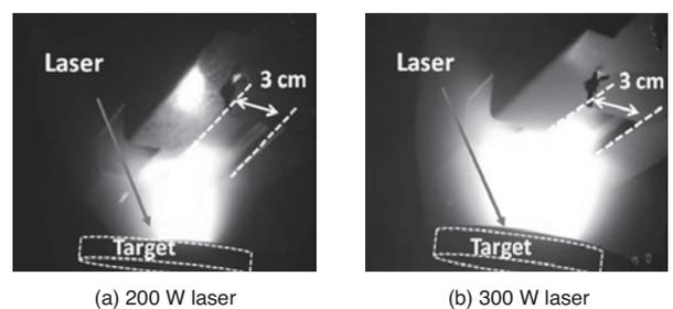
Fig. 4. Comparison of plasma plume between 200 W laser and 300 W laser
