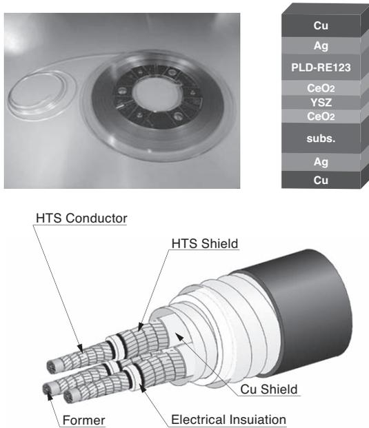
Fig. 1. Architecture of coated conductor and HTS cable
