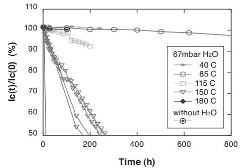
**Fig. 10.** Time duration of  $I_c$  property under humid conditions
