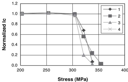
Fig. 13. Tensile stress effect on the  $I_c$  property of Clad-PLD conductor
