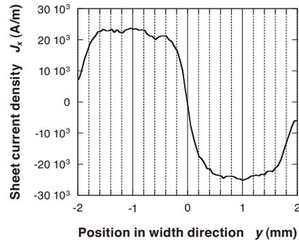
Fig. 15.  $I_c$  distribution of narrow conductor by mechanical slitting method
