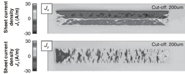
Fig. 14. Evaluation of current distribution of Clad-PLD conductor by hall probe method
