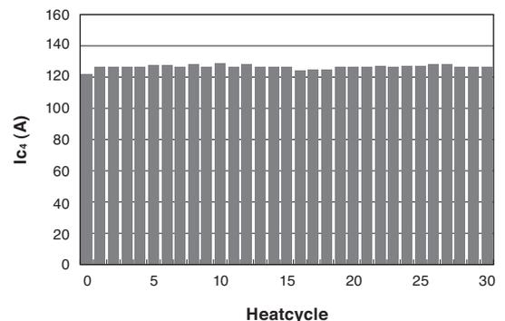
**Fig. 11.** Dependence of heat cycle on  $I_c$  (room temperature to liquid N<sub>2</sub> temperature)
