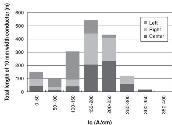
Fig. 8.  $I_c$  distributions of 4 mm-width Clad-PLD conductors
