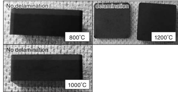
Photo 5. Appearance of sintering in low temperature
