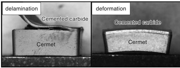
Photo 3. Appearance of delamination and deformation
