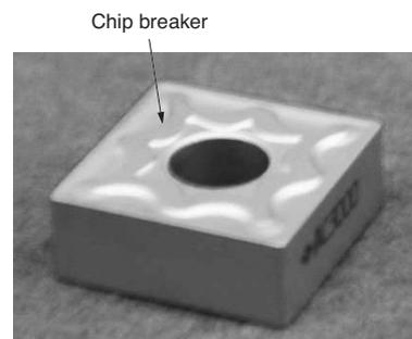
**Photo 2.** Cutting tool of cemented carbide
