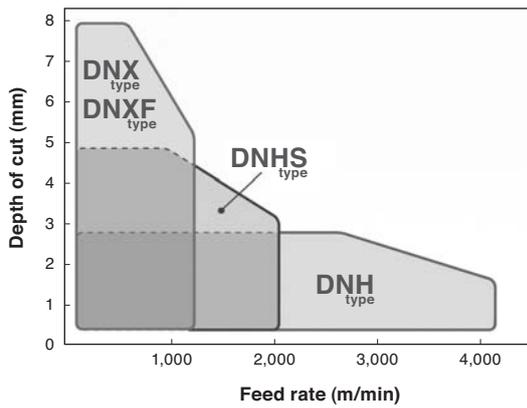
Fig. 6. Application Range of DNX-Series Cutters
