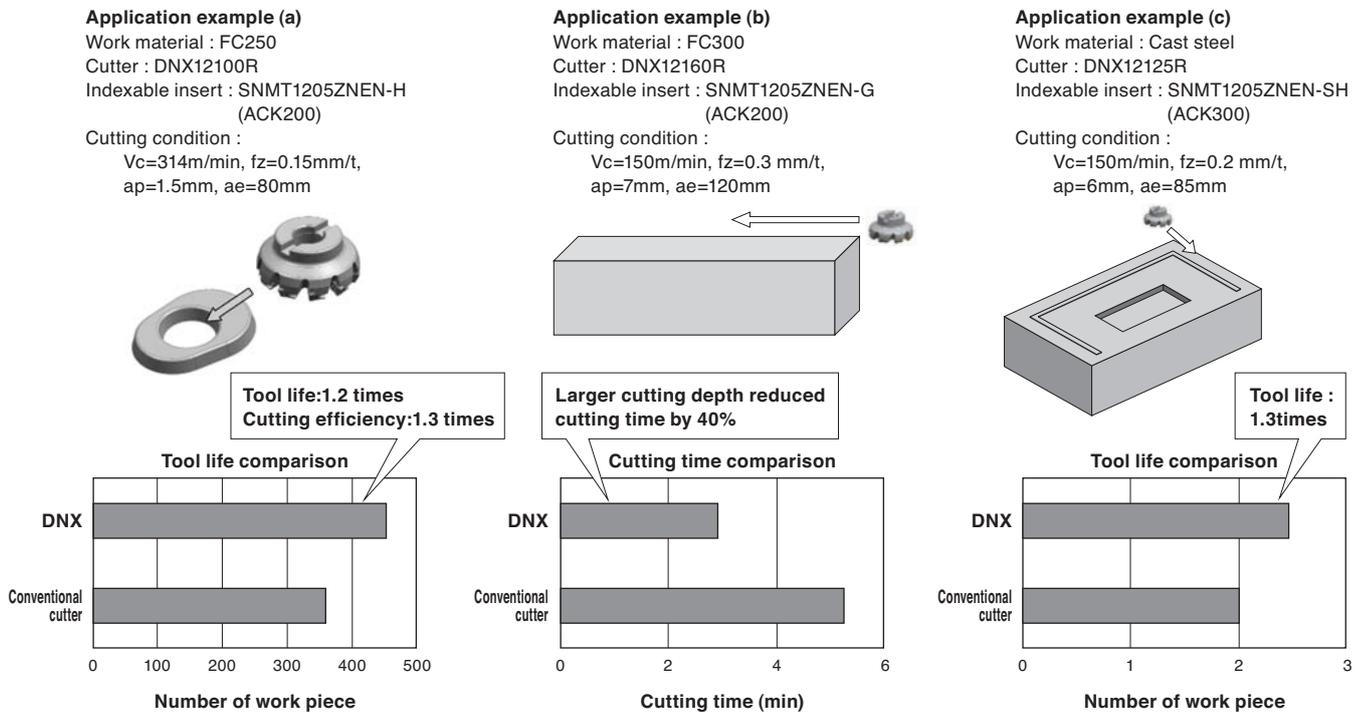
Fig. 8. Application Examples of DNX-Series Cutters
