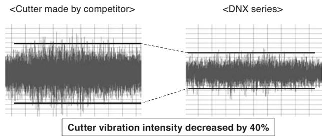
Fig. 4. Cutter Vibration Intensity Comparison
