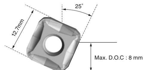
Fig. 1. DNX Series Indexable Insert Size and Cutting Edge Specifications
