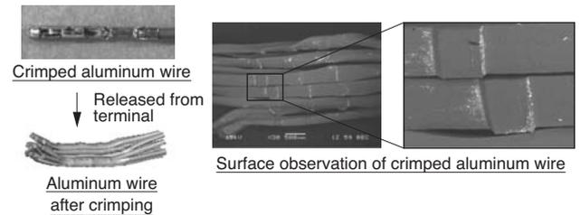
**Fig. 15.** Crimped wire surface observation
