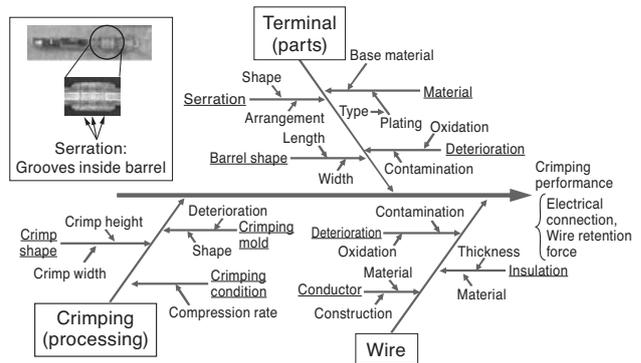
**Fig. 11.** Cause and effect diagram regarding crimping properties
