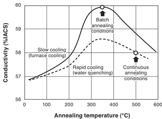
Fig. 4. Effect of annealing conditions on conductivity
