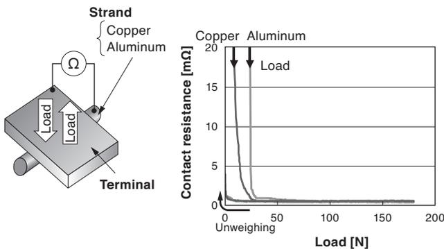
**Fig. 9.** Load and contact resistance
