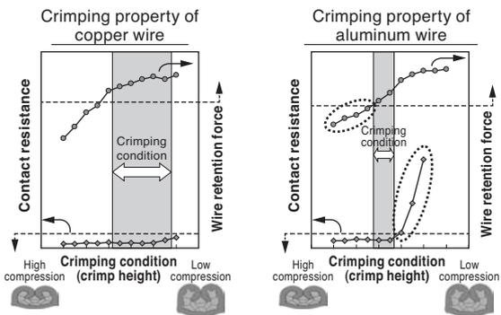
**Fig. 10.** Crimping strength, contact resistance and wire retention force
