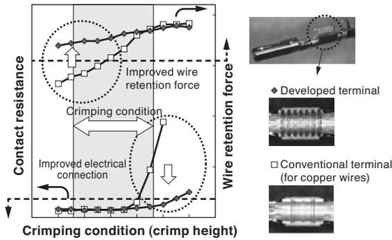
**Fig. 17.** Crimping properties of terminal for aluminum wire
