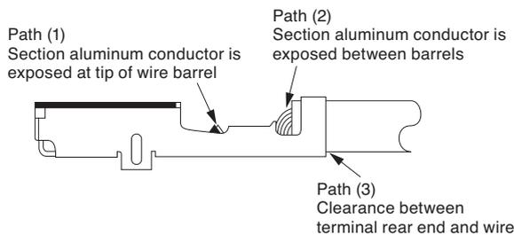
**Fig. 21.** Moisture intrusion paths into crimped section of aluminum wire
