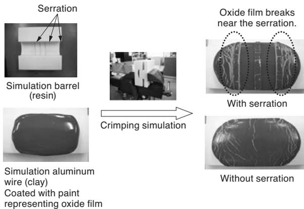
**Fig. 13.** Simulation test using clay
