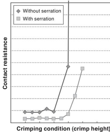
**Fig. 12.** Crimping properties of terminal with and without serration
