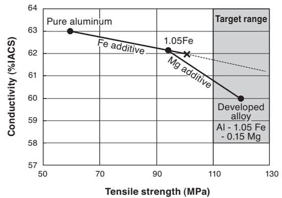
**Fig. 3.** Component and performance of developed alloy
