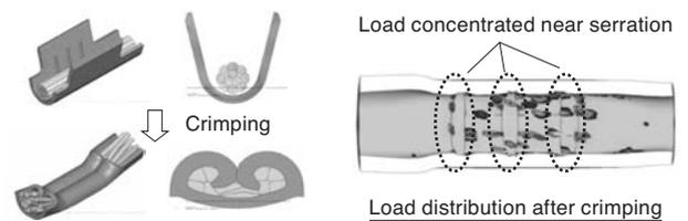
**Fig. 14.** Crimping simulation using CAE
