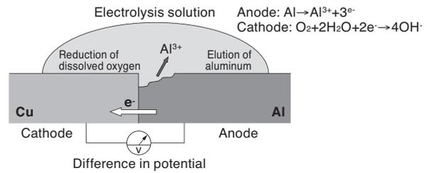
**Fig. 18.** Bimetallic corrosion of copper and aluminum
