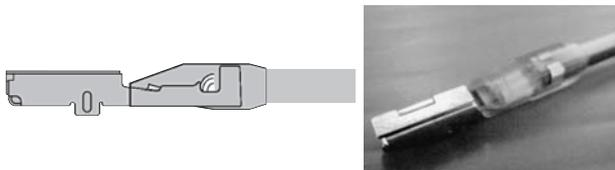
**Fig. 22.** Mold structure of aluminum wire crimping section
