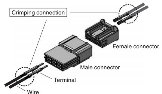
Fig. 7. Connectors and crimped wires
