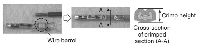
Fig. 8. Crimping connection
