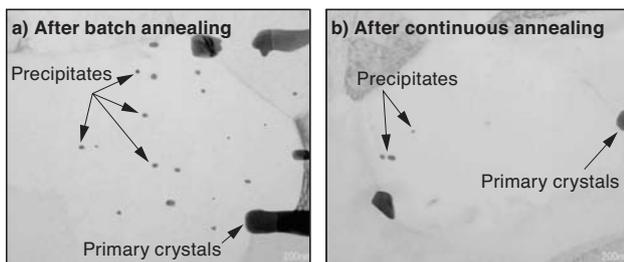
Fig. 5. Difference in precipitation due to different annealing methods
