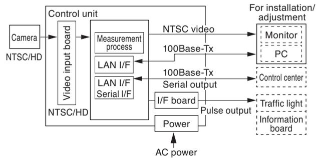
Fig. 2. Equipment configuration
