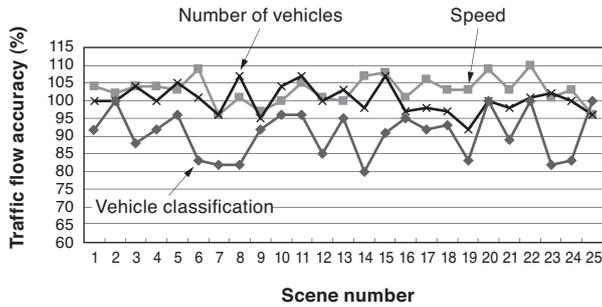
Fig. 4. Traffic flow measurement accuracy of NTSC camera
