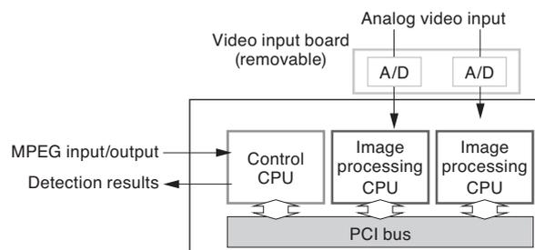
Fig. 3. Processing board configuration
