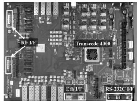
Photo 1. MindSpeed Transcde 4000 test board
