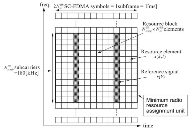
Fig. 4. Minimum radio resource assignment unit (localized type)<sup>(1)</sup>
