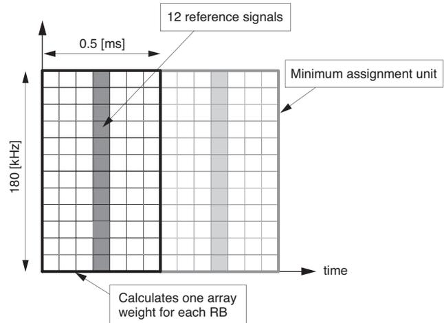
Fig. 7. RB based array weight
