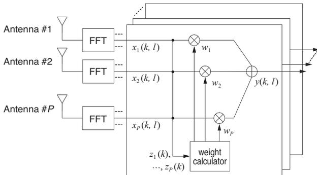
Fig. 2. Array antenna for LTE uplink channels
