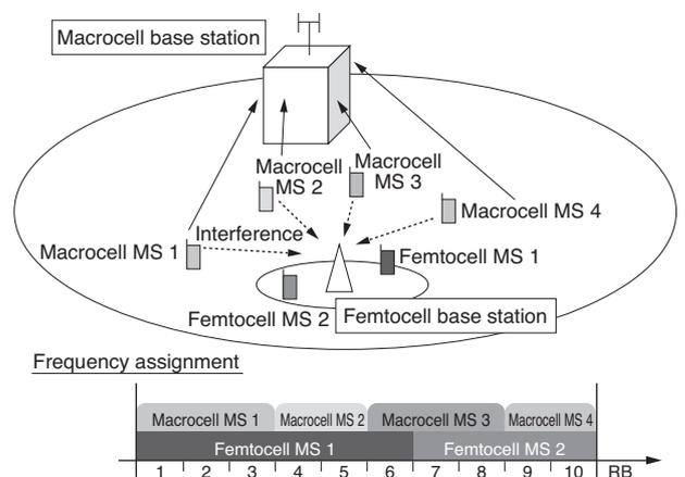
Fig. 5. Frequency assignment and interference from macrocell mobile stations (MS)
