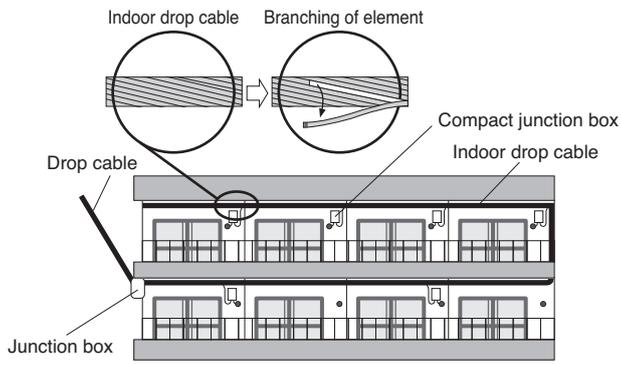
Fig. 2. Example of wiring in outer wall of MDUs
