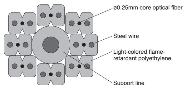
**Fig. 1.** Structure of MDU indoor drop cable
