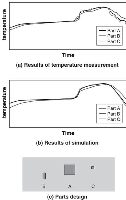
Fig. 8. Temperature of parts in reflow furnace
