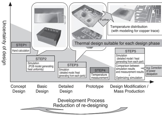
Fig. 2. Thermal design process
