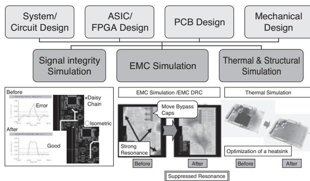
Fig. 1. Simulation-based design method
