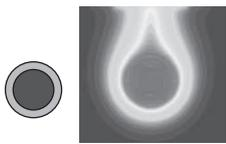
(a) Pattern diagram of round-shaped electric wire and temperature distribution
