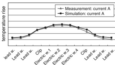
(d) Temperature of electric wire with the new structure Comparison between measurement results and simulation results
