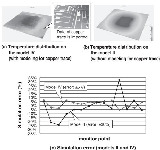
**Fig. 4.** Modeling example of copper trace
