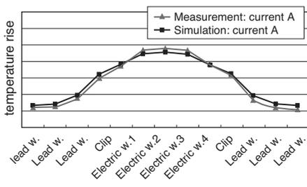
(c) Temperature of round-shaped wire Comparison between measurement results and simulation results
