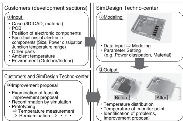
Fig. 3. Thermal design flow
