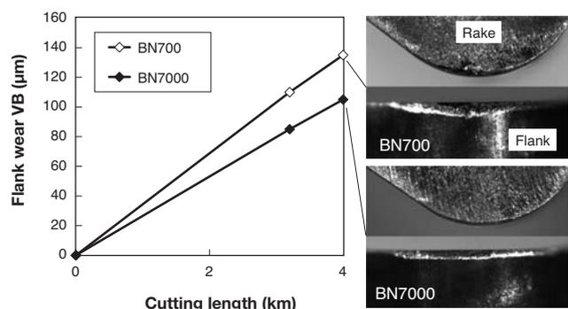
Fig. 3. Result of cutting test of ferrous PM
