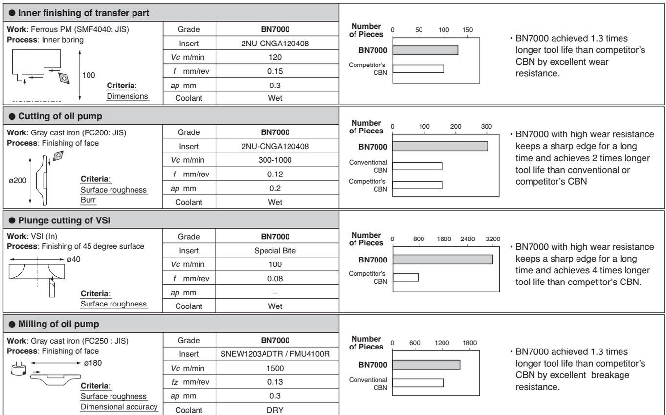
Fig. 8. Examples of machining by BN7000
