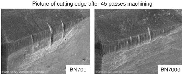
Photo 2. Comparison after the milling test on cast iron
