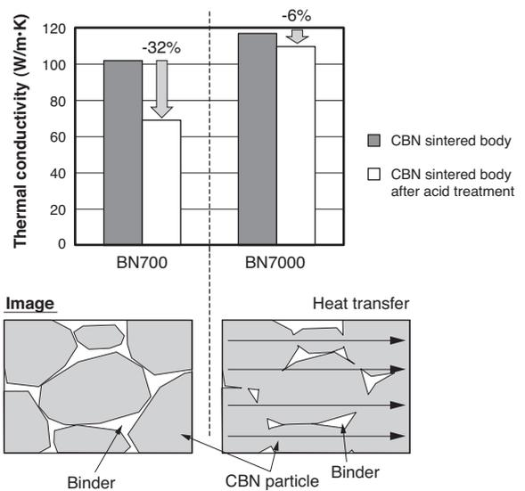
Fig. 5. Thermal conductivity of CBN compact
