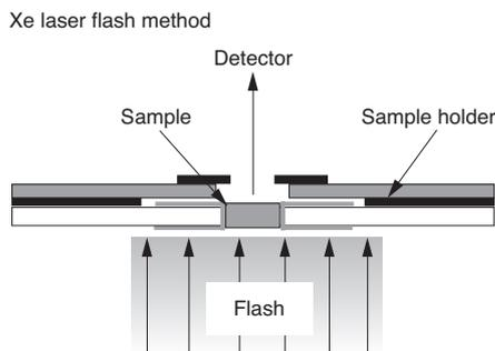
Fig. 4. Thermal conductivity measurement
