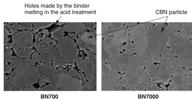
Photo 1. Microstructure of CBN compact after acid treatment
