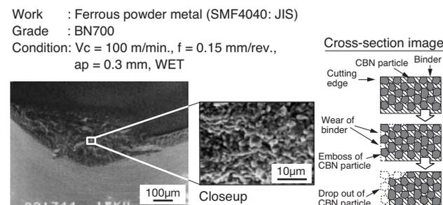
Fig. 2. Tool failures in ferrous PM machining
