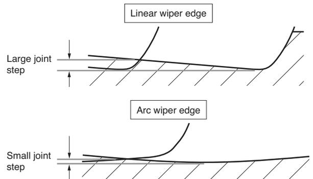
Fig. 4. linear and arc wiper edges
