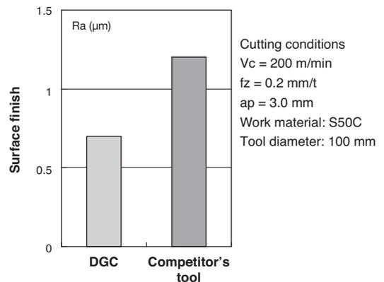
Fig. 5. Quality of machined surface
