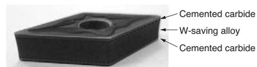
Photo 2. Appearance of composite structure tool
