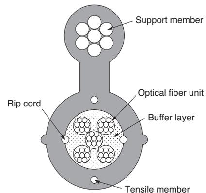
Fig. 2.  $\phi 0.5\text{mm}$  optical fiber aerial cable
