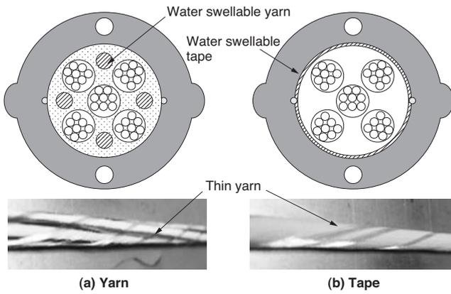
Fig. 5. Water blocking material composition and cable cores
