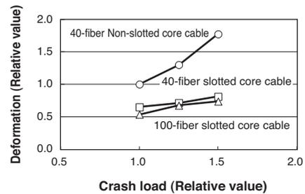
**Fig. 8.** Deformation in the crash examination
