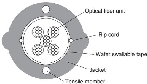
Fig. 3. Cross section of 40-fiber non-slotted core cable
