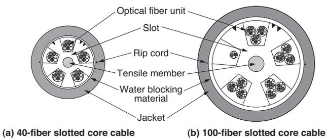
**Fig. 7.** Cross section of slotted core cables
