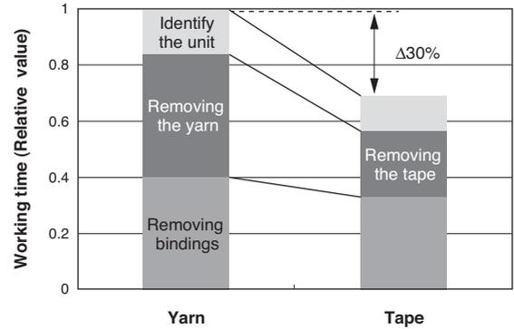
Fig. 6. Comparison of working time
