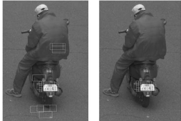
Photo 4. Example of the result of plate detection
