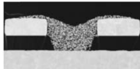
Photo 3. Cross section of \phi 40\mu\text{m} blind via using the conductive paste
