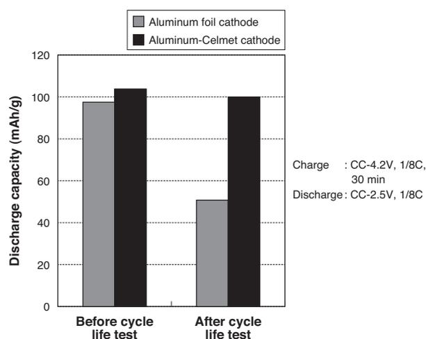
Fig. 6. Changes in Discharge Capacity of the Lithium Ion Battery Incorporating Aluminum-Celmet before and after Cycle Life Test at 60°C
