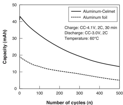
Fig. 5. Change in the Capacity of Lithium Ion Battery Incorporating Aluminum-Celmet under 60°C
