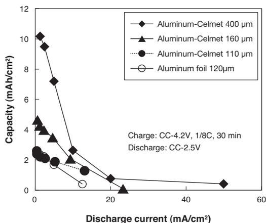
**Fig. 3.** Discharge Rate Property of Lithium Ion Batteries Incorporating Aluminum-Celmet
