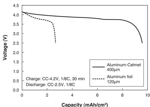
**Fig. 2.** Discharge Property of Lithium Ion Batteries Incorporating Aluminum-Celmet at a Charge-Discharge Rate of 1/8C
