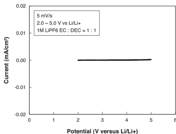
Fig. 1. Aluminum-Celmet Corrosion Resistance
