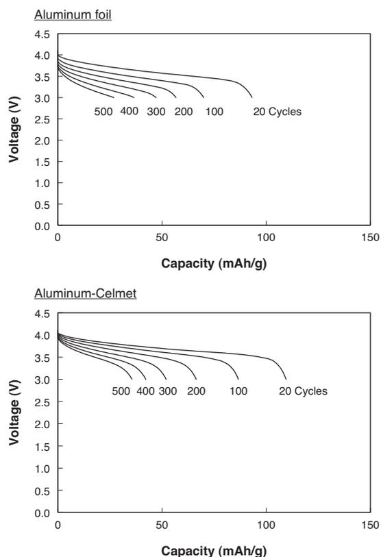
Fig. 4. Changes in the Discharge Capacity of Lithium Ion Batteries Incorporating Aluminum-Celmet under 60°C after Different Numbers of Charge-Discharge Cycles
