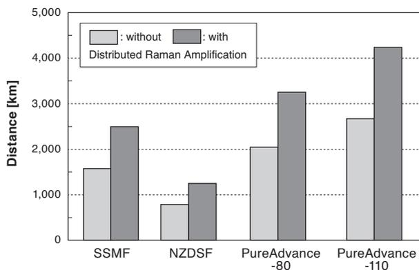
**Fig. 7.** Maximum transmission distance for a 80 km-span link with 100 Gb/s DP-QPSK format
