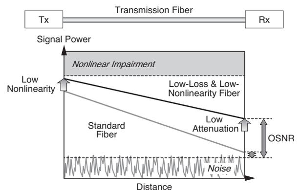
**Fig. 1.** Schematic of OSNR improvement by low attenuation and low nonlinearity of fiber
