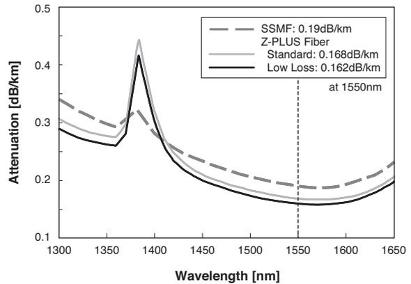
Fig. 2. Attenuation spectra of SSMF, Z-PLUS Fiber and Z-PLUS Fiber LL
