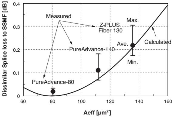
**Fig. 4.** Splice loss between low-loss and low-nonlinearity PSCFs and SSMF
