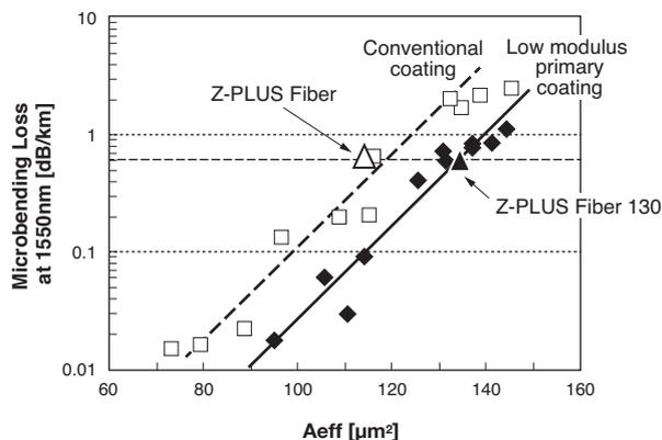
Fig. 3. Microbending loss for fibers with low Young's modulus primary and conventional coatings
