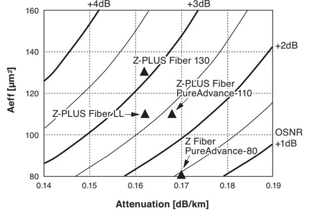
**Fig. 5.** Relative OSNR normalized to that for SSMF in a 1500km-reach transmission link with 80km-span
