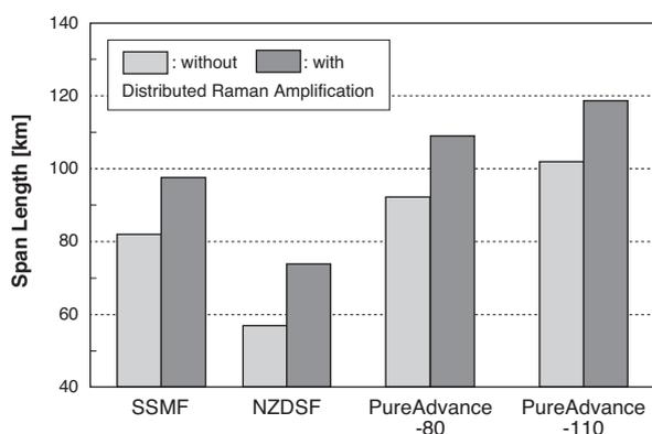
**Fig. 6.** Maximum span length for a 1500km transmission link with 100 Gb/s DP-QPSK format
