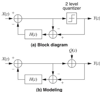
Fig. 6. Block diagram and modeling of BP-DSM
