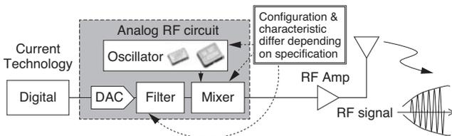
**Fig. 2.** Conventional radio transmitter
