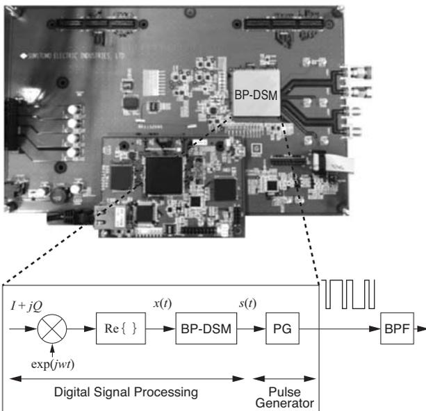
Fig. 11. Prototype of circuit board for 1-bit digital RF transmitter
