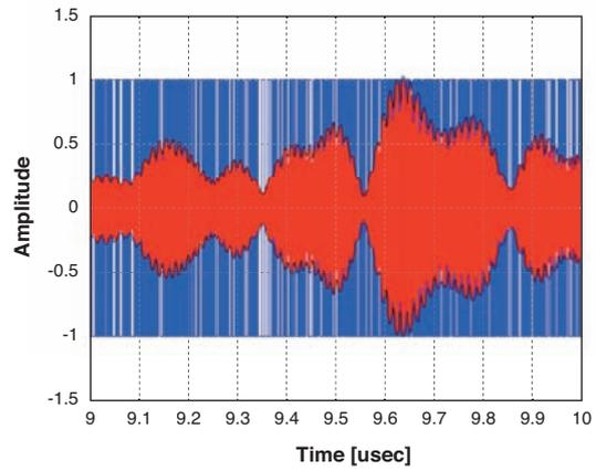
Fig. 7. Input-output waveforms of BP-DSM
