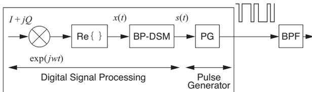
Fig. 5. Block diagram of 1-bit digital RF transmitter
