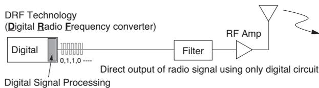
**Fig. 3.** 1-bit digital RF transmitter
