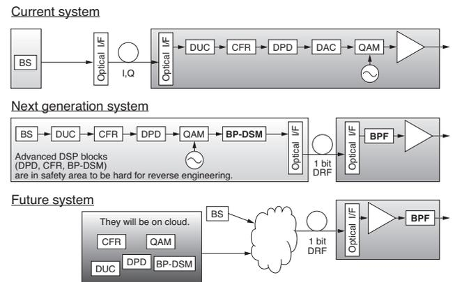
**Fig. 4.** Use of 1-bit digital RF transmitter with optical link
