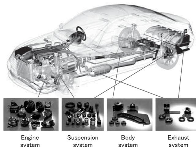
Fig. 1. Anti-vibration rubber products for vehicles
