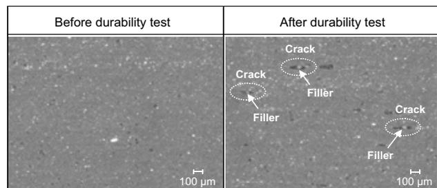
Fig. 3. Progress of cracks in the rubber
