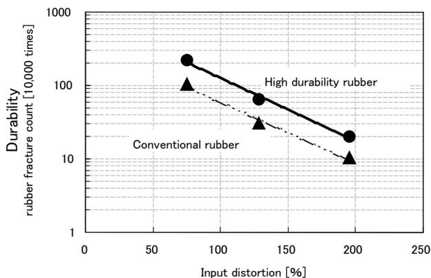
Fig. 5. Durability input distortion dependence
