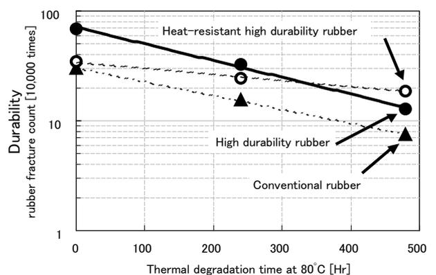
Fig. 7. Durability of high durability rubber after thermal degradation
