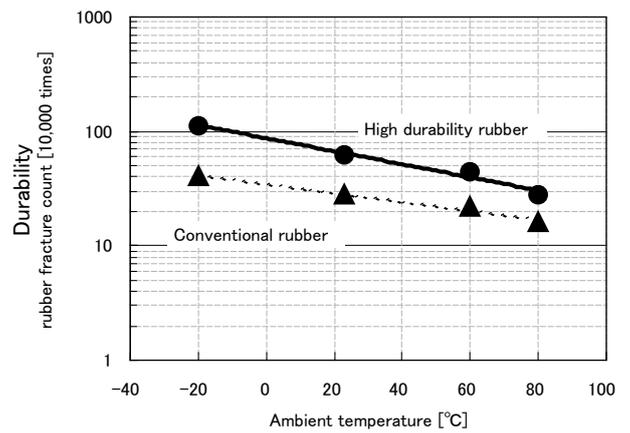
Fig. 6. Durability of high durability rubber at each ambient temperature
