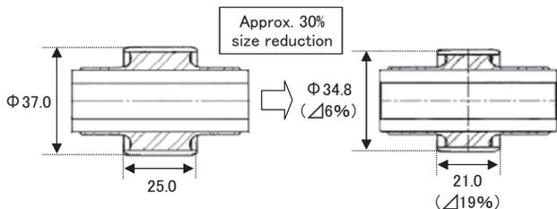
Fig. 8. Product shape used in the durability test
