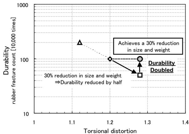
Fig. 2. Rubber input distortion and durability due to decrease in size
