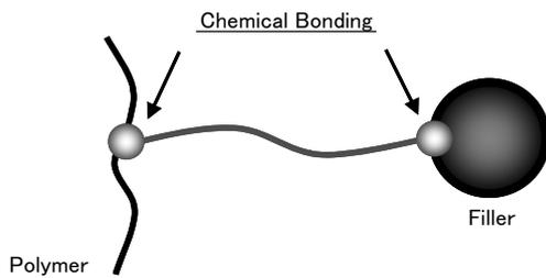
Fig. 4. Reinforcing the filler interface
