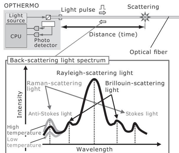
Fig. 1. OPTHERMO measurement mechanism
