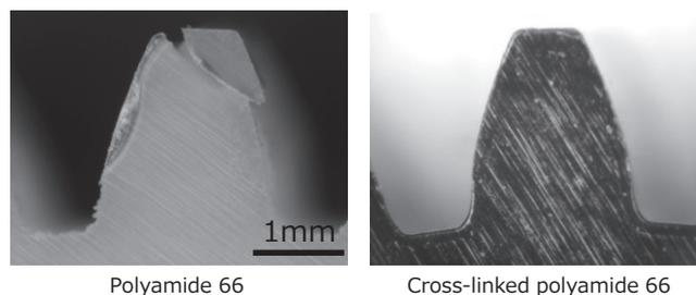
Photo 1. Gear tooth tip after the fatigue test
