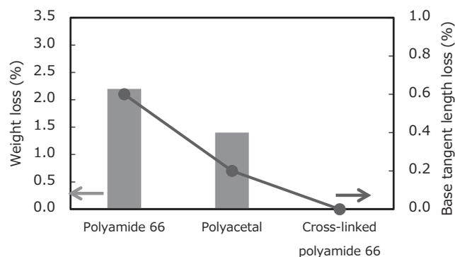
Fig. 3. Results of the gear fatigue test
