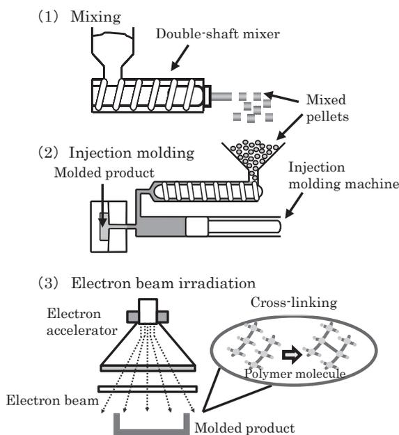
Fig. 1. Manufacturing process of electron beam-irradiated cross-linked molded products
