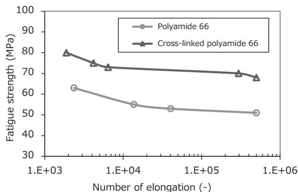
Fig. 2. Measurement results of dumbbell fatigue strength
